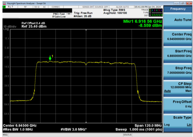
Plot 7-727. LPI Power Spectral Density Plot SDM Primary Antenna 3c (80MHz 802.11ax RU996 (UNII Band 8) – Ch. 199)
