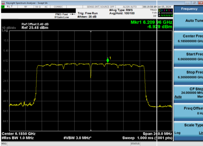
Plot 7-640. LPI Power Spectral Density Plot SDM Primary Antenna 3a (160MHz 802.11ax RU996x2 (UNII Band 5) – Ch. 47)
