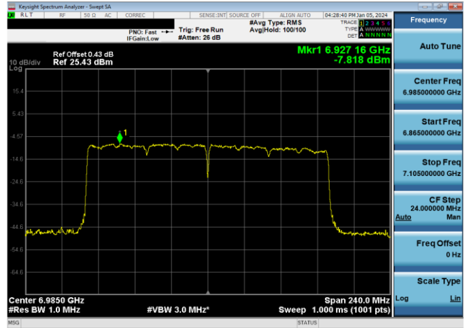
Plot 7-608. LPI Power Spectral Density Plot Antenna 1b (160MHz 802.11ax RU996x2 (UNII Band 8) – Ch. 207)
