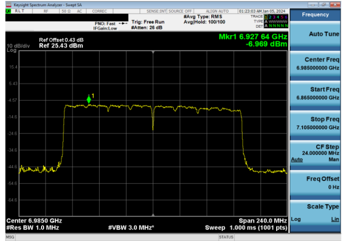
Plot 7-544. LPI Power Spectral Density Plot Antenna 3a (160MHz 802.11ax RU996x2 (UNII Band 8) – Ch. 207)
