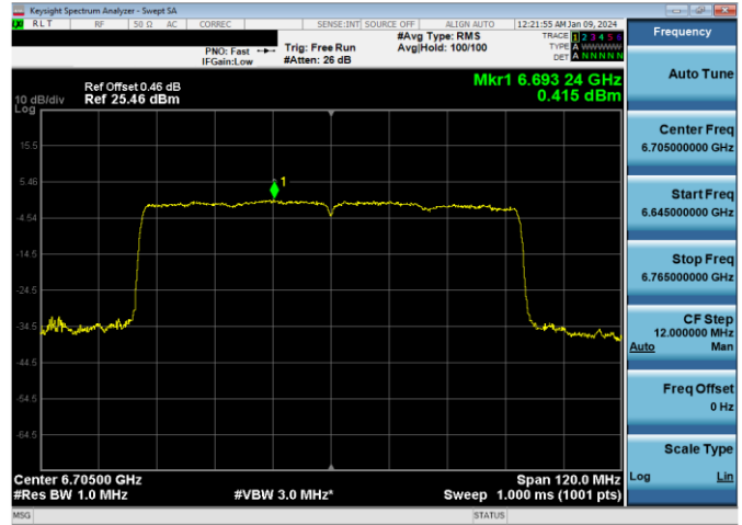
Plot 7-252. SP Power Spectral Density Plot Antenna 3a (80MHz 802.11ax RU996 (UNII Band 7) – Ch. 151)
