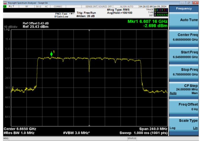
Plot 7-288. SP Power Spectral Density Plot Antenna 1b (160MHz 802.11ax RU996x2 (UNII Band 7) – Ch. 143)
