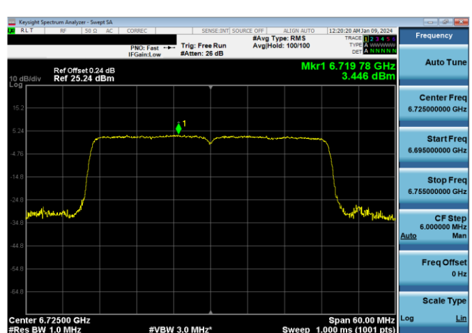
Plot 7-248. SP Power Spectral Density Plot Antenna 3a (40MHz 802.11ax RU484 (UNII Band 7) – Ch. 155)
