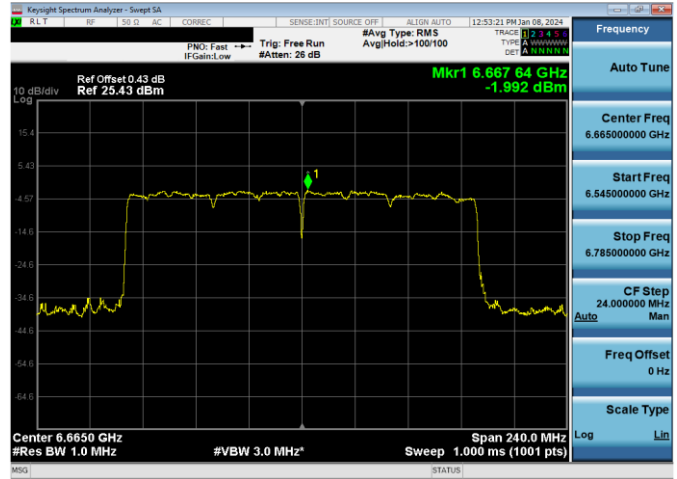
Plot 7-224. SP Power Spectral Density Plot Antenna 3c (160MHz 802.11ax RU996x2 (UNII Band 7) – Ch. 143)
