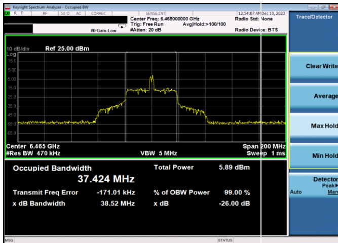
Plot 7-26. 26dB & 99% Bandwidth Plot Antenna 3c (80MHz 802.11ax RU26 (UNII Band 6) – Ch. 103)
