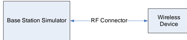
Figure 8-2 Power Measurement Setup
