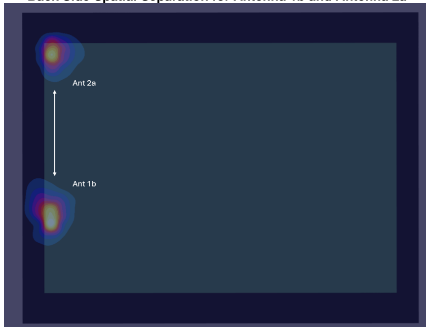
Figure 11-7 Back Side Spatial Separation for Antenna 1b and Antenna 2a
