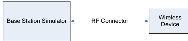
Figure 8-1 Power Measurement Setup
