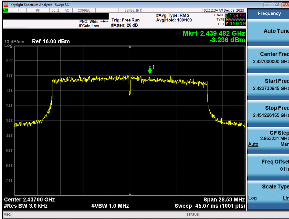
Plot 7-153. Power Spectral Density Plot CDD Antenna 3a (802.11ax (SU - 2.4GHz) – Ch. 6) – MCS4
