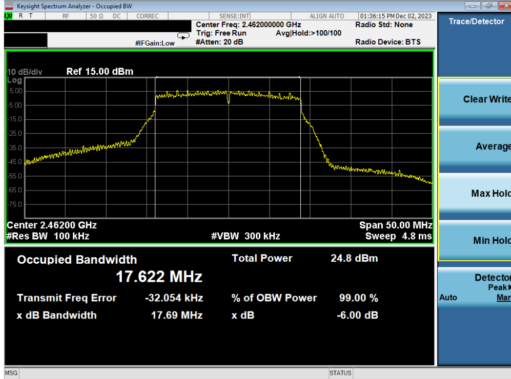
Plot 7-15. 6 dB BW and 99% OBW Plot Antenna 3a (802.11n (2.4GHz) – Ch. 11) – MCS4
