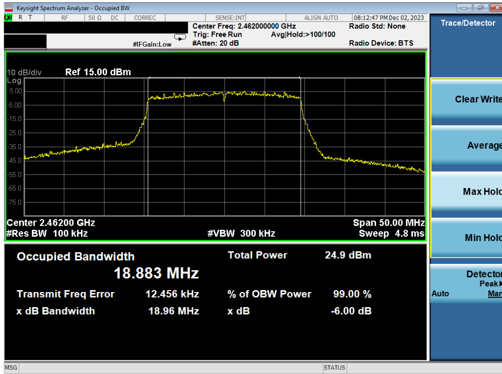
Plot 7-48. 6 dB BW and 99% OBW Plot Antenna 1a (802.11ax (SU - 2.4GHz) – Ch. 11) – MCS4
