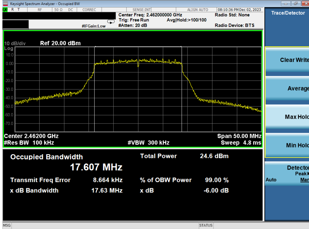
Plot 7-45. 6 dB BW and 99% OBW Plot Antenna 1a (802.11n (2.4GHz) – Ch. 11) – MCS4
