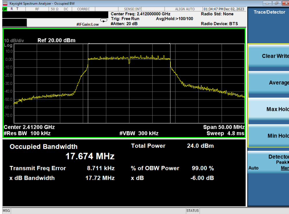
Plot 7-13. 6 dB BW and 99% OBW Plot Antenna 3a (802.11n (2.4GHz) – Ch. 1) – MCS4
