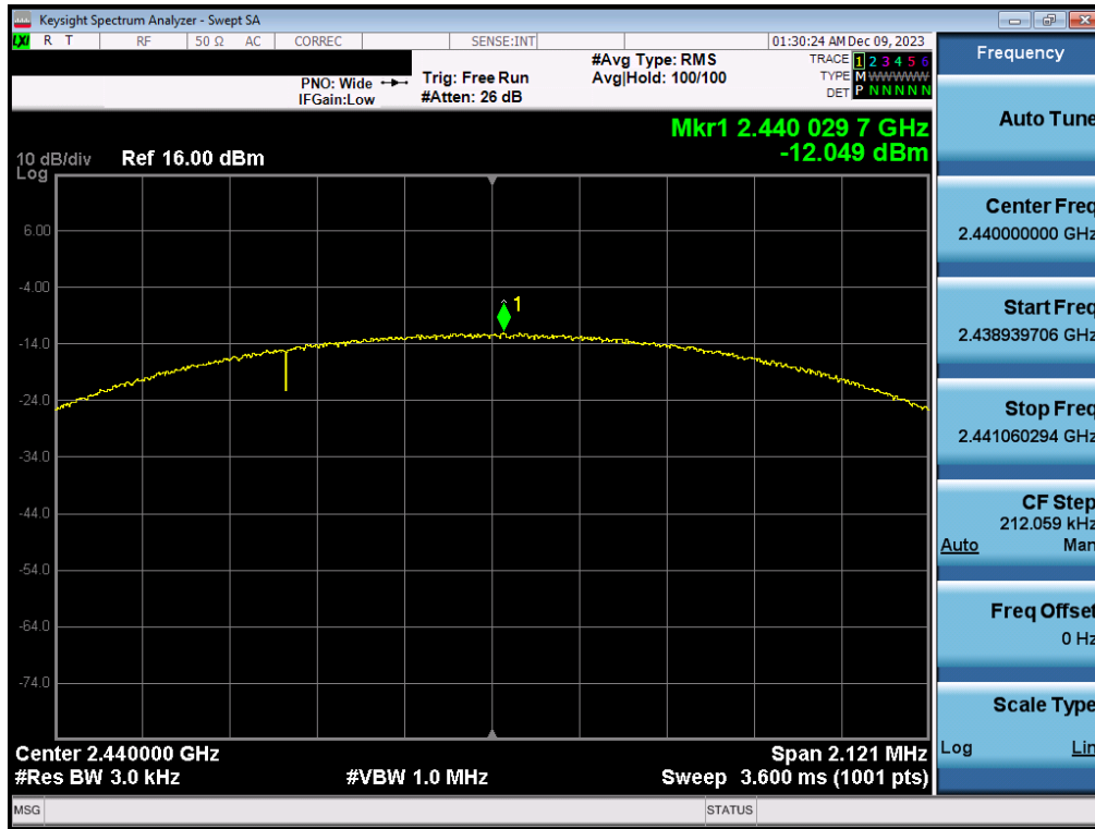
Plot 7-57. Power Spectral Density Plot Antenna 3a (Bluetooth (LE), 2Mbps, iPA – Ch. 19)
