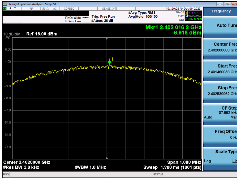
Plot 7-43. Power Spectral Density Plot Antenna 3a (Bluetooth (LE), 1Mbps, iPA – Ch. 0)
