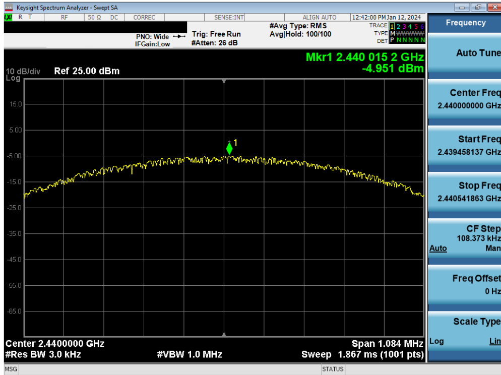
Plot 7-39. Power Spectral Density Plot Antenna 3a (Bluetooth (LE), 1Mbps, ePA – Ch. 19)
