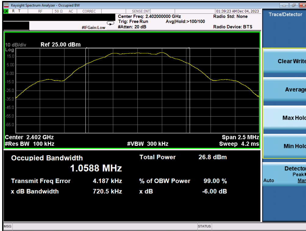
Plot 7-7. 6dB BW & 99% OBW Plot Antenna 1a (Bluetooth (LE), 1Mbps, ePA – Ch. 0)
