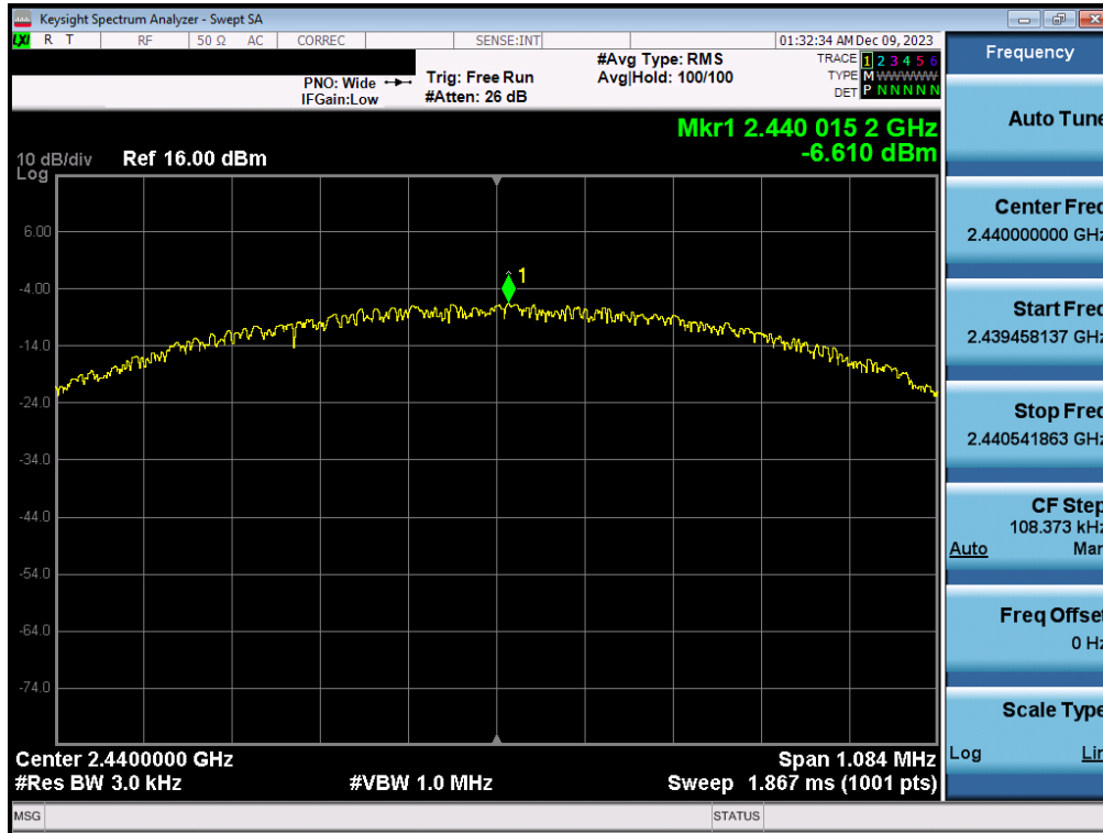
Plot 7-17. Power Spectral Density Plot Antenna 3a (Bluetooth (LE), 1Mbps, iPA – Ch. 19)
