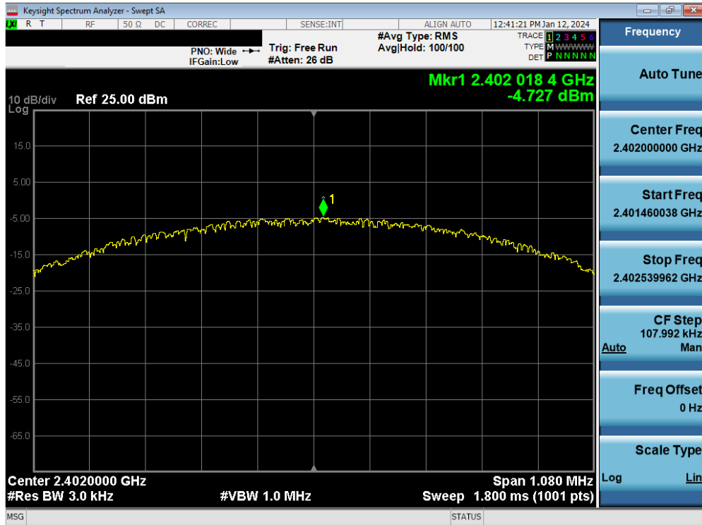
Plot 7-37. Power Spectral Density Plot Antenna 3a (Bluetooth (LE), 1Mbps, ePA – Ch. 0)
