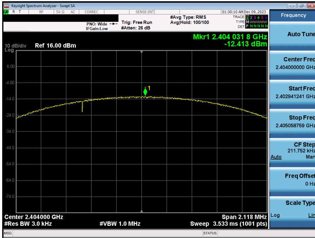
Plot 7-55. Power Spectral Density Plot Antenna 3a (Bluetooth (LE), 2Mbps, iPA – Ch. 1)
