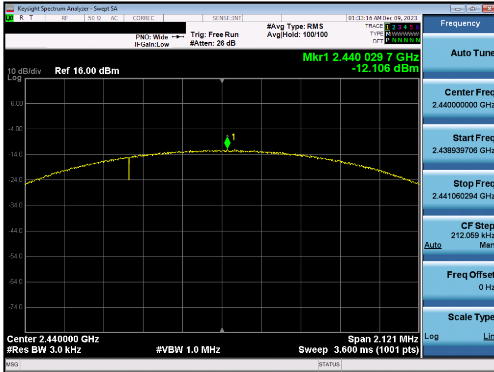
Plot 7-23. Power Spectral Density Plot Antenna 3a (Bluetooth (LE), 2Mbps, iPA – Ch. 19)
