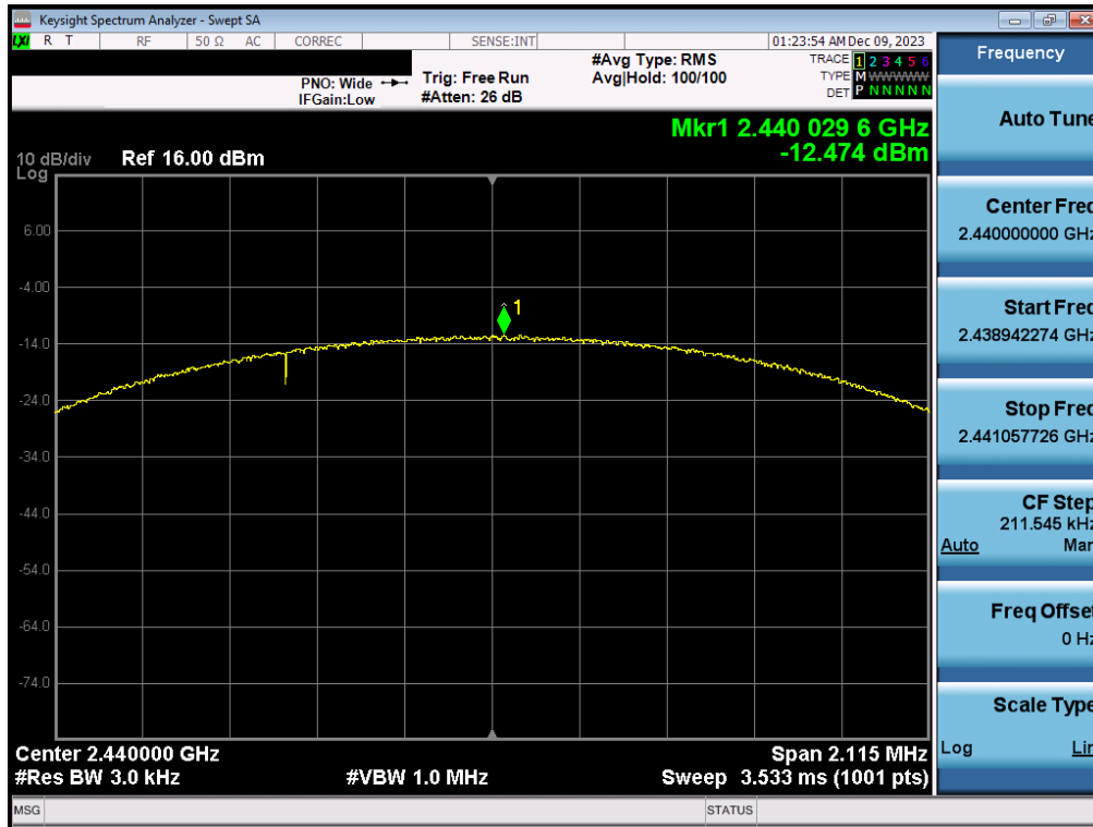
Plot 7-35. Power Spectral Density Plot Antenna 1a (Bluetooth (LE), 2Mbps, iPA – Ch. 19)
