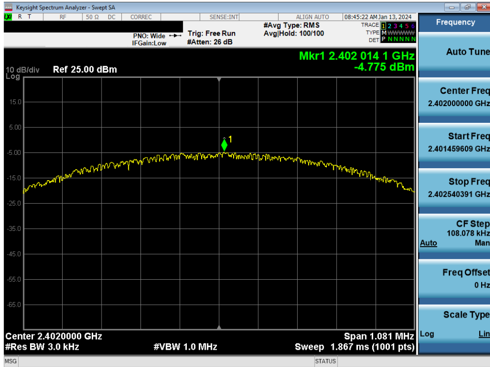
Plot 7-25. Power Spectral Density Plot Antenna 1a (Bluetooth (LE), 1Mbps, ePA – Ch. 0)
