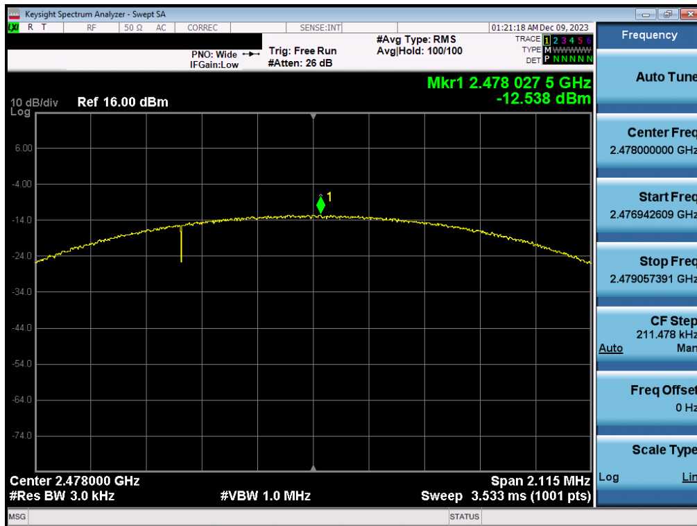
Plot 7-60. Power Spectral Density Plot Antenna 1a (Bluetooth (LE), 2Mbps, iPA – Ch. 38)
