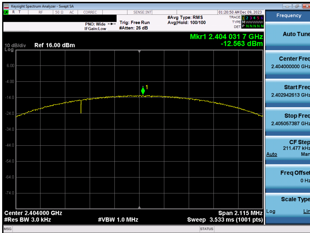
Plot 7-56. Power Spectral Density Plot Antenna 1a (Bluetooth (LE), 2Mbps, iPA – Ch. 1)
