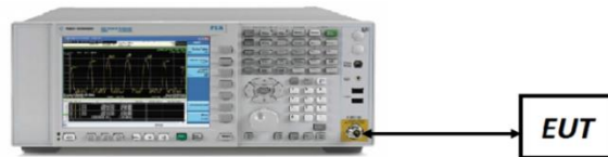
Figure 7-4. Test Instrument & Measurement Setup
