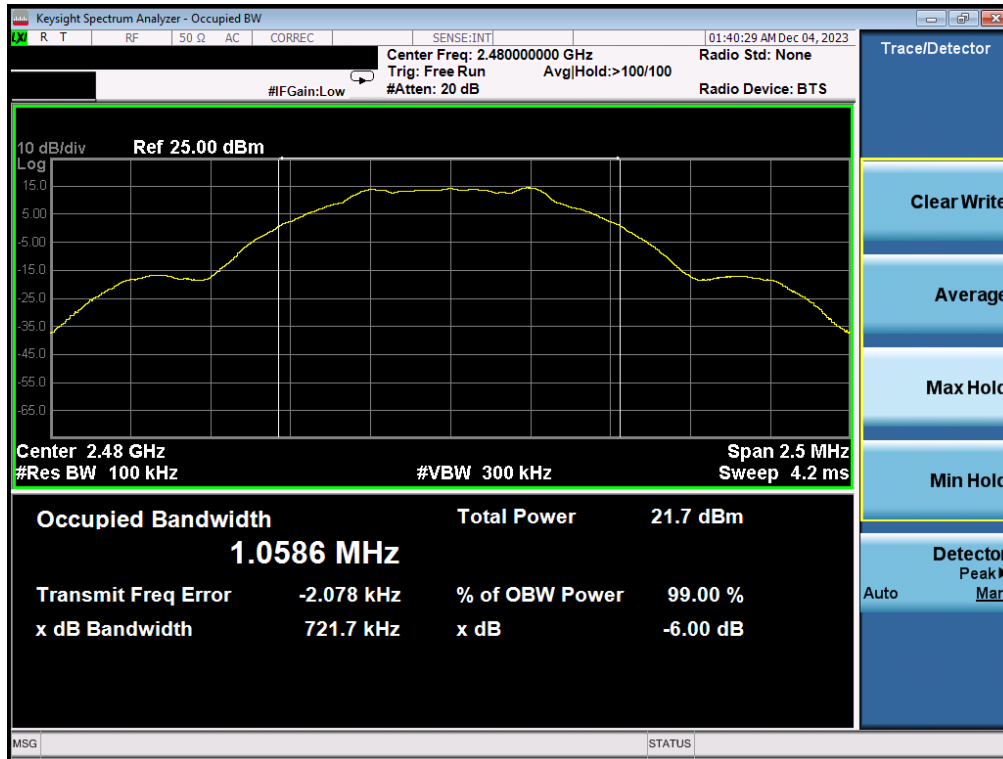
Plot 7-9. 6dB BW & 99% OBW Plot Antenna 1a (Bluetooth (LE), 1Mbps, ePA – Ch. 39)
