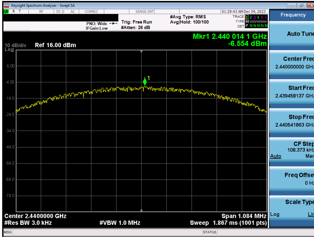
Plot 7-45. Power Spectral Density Plot Antenna 3a (Bluetooth (LE), 1Mbps, iPA – Ch. 19)
