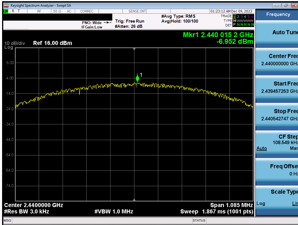
Plot 7-29. Power Spectral Density Plot Antenna 1a (Bluetooth (LE), 1Mbps, iPA – Ch. 19)
