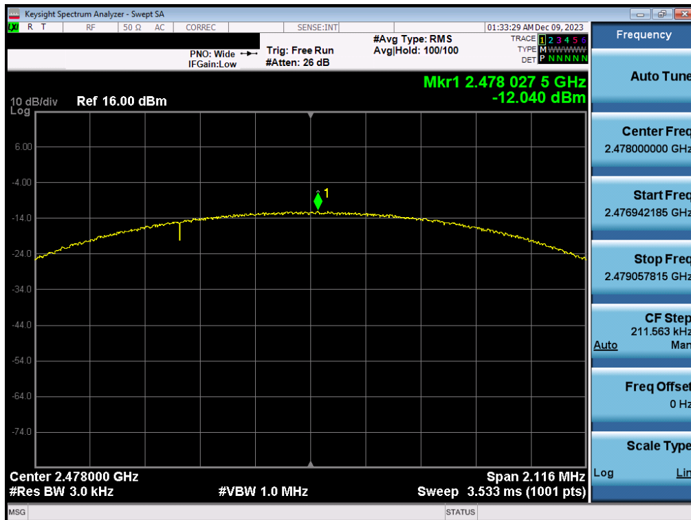
Plot 7-24. Power Spectral Density Plot Antenna 3a (Bluetooth (LE), 2Mbps, iPA – Ch. 38)
