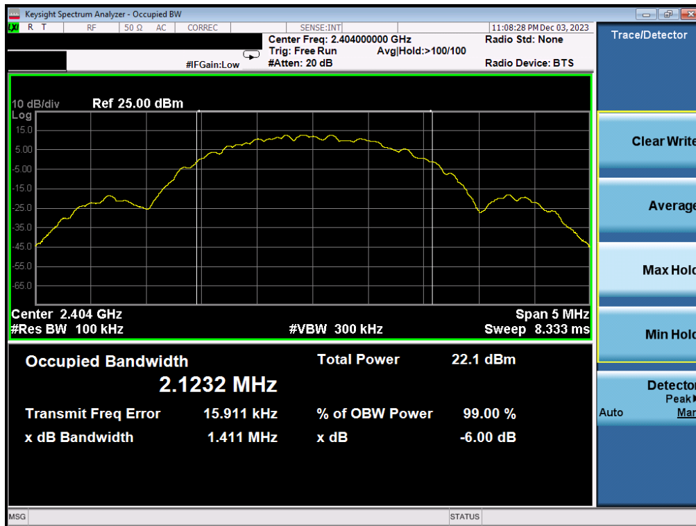
Plot 7-4. 6dB BW & 99% OBW Plot Antenna 3a (Bluetooth (LE), 2Mbps, ePA – Ch. 39)
