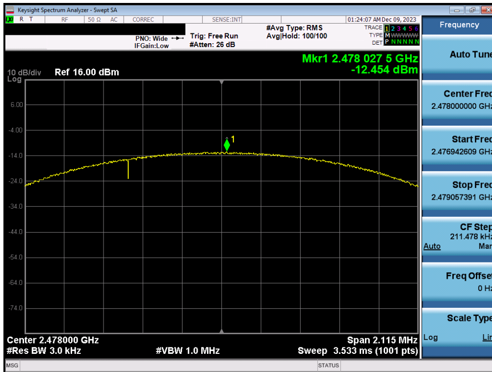
Plot 7-36. Power Spectral Density Plot Antenna 1a (Bluetooth (LE), 2Mbps, iPA – Ch. 38)
