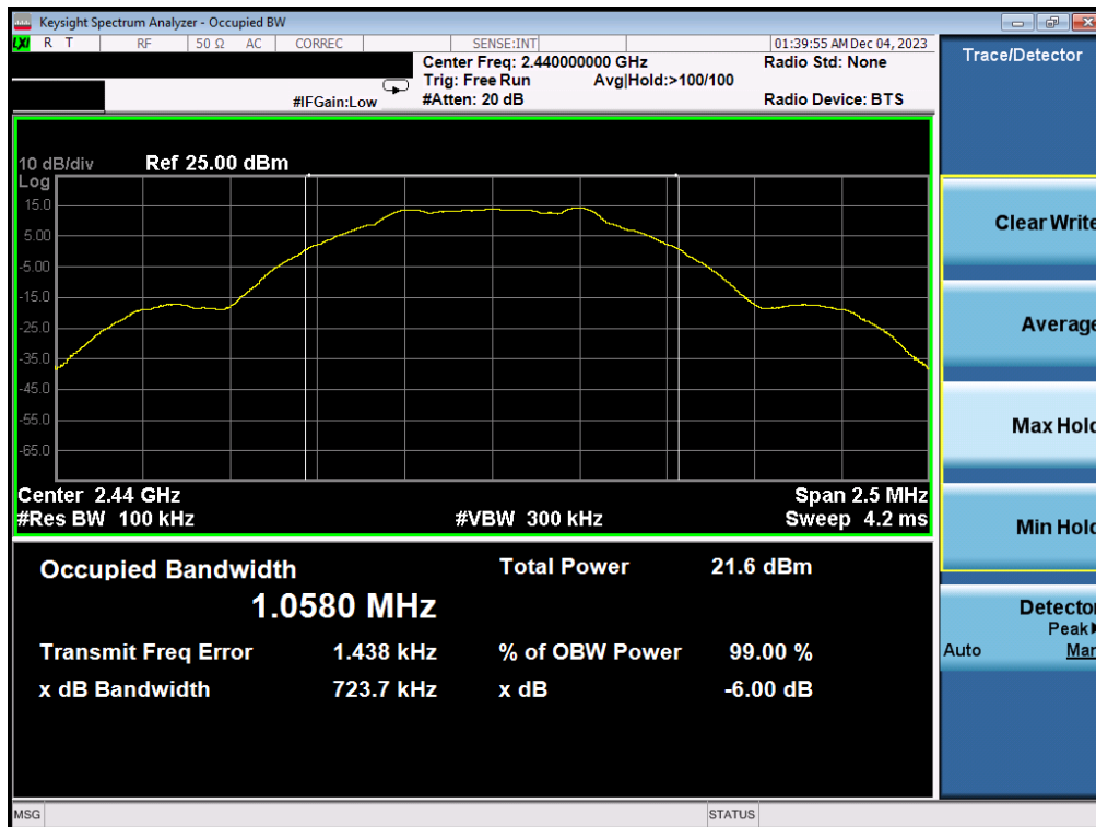
Plot 7-8. 6dB BW & 99% OBW Plot Antenna 1a (Bluetooth (LE), 1Mbps, ePA – Ch. 19)
