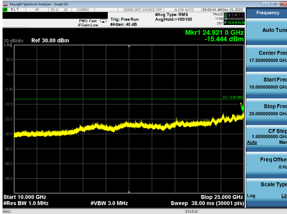
Plot 7-74. Conducted Spurious Plot Antenna 3a (Bluetooth (HDR4), 4 Mbps, ePA – Ch. 73)
