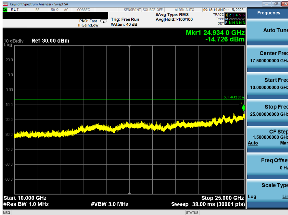
Plot 7-80. Conducted Spurious Plot Antenna 1a (Bluetooth (HDR4), 4 Mbps, ePA – Ch. 73)
