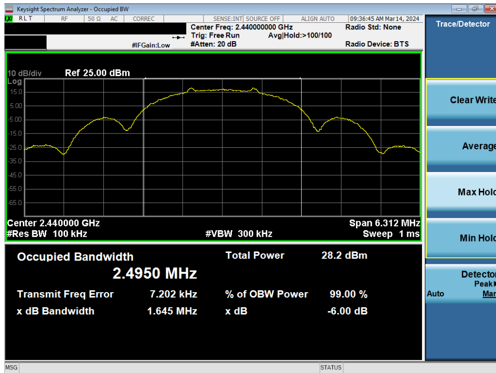
Plot 7-2. 6dB BW & 99% OBW Antenna 3a (802.15.4, Ch. 18)
