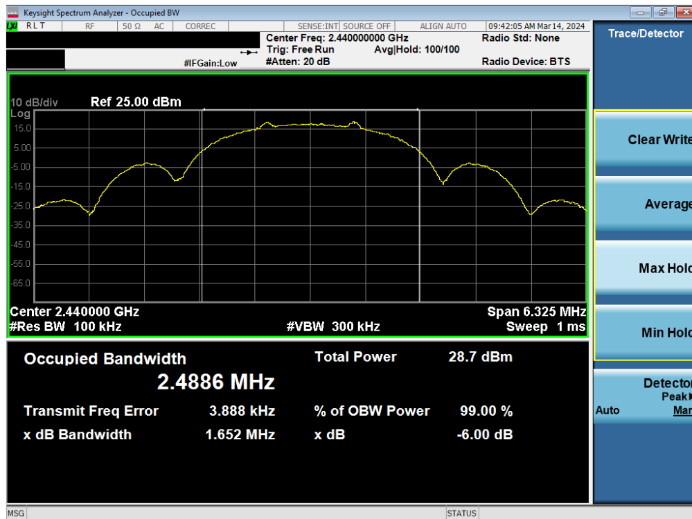
Plot 7-5. 6dB BW & 99% OBW Antenna 1a (802.15.4, Ch. 18)
