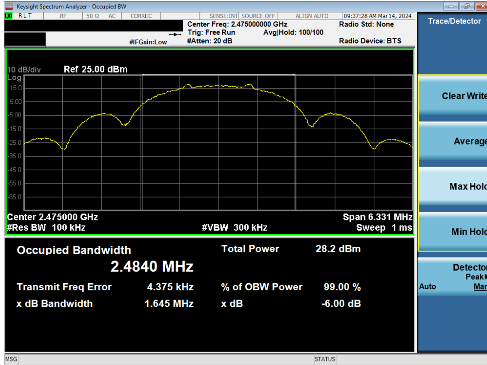
Plot 7-3. 6dB BW & 99% OBW Antenna 3a (802.15.4, Ch. 25)
