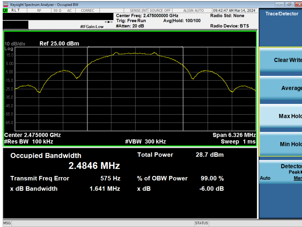
Plot 7-6. 6dB BW & 99% OBW Antenna 1a(802.15.4, Ch. 25)
