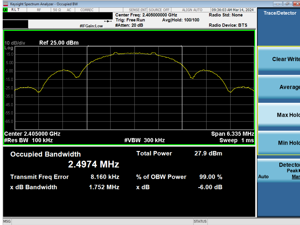
Plot 7-1. 6dB BW & 99% OBW Antenna 3a (802.15.4, Ch. 11)
