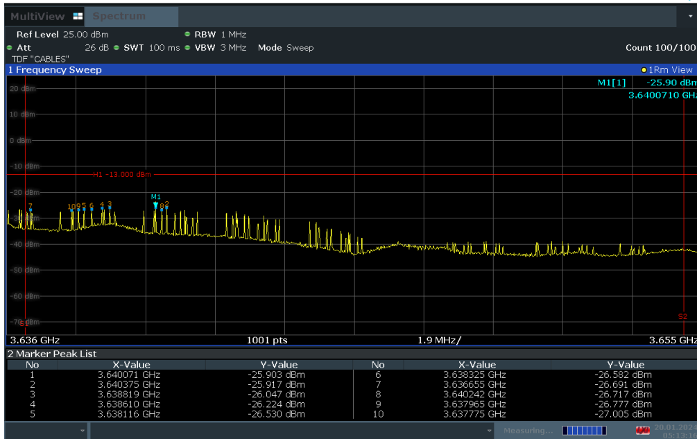
Plot 7-152. Channel Edge Plot (LTE Band 48 - 15MHz QPSK - Mid Channel)
