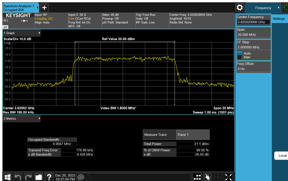
Plot 7-36. Occupied Bandwidth Plot (NR Band n48 - 10MHz CP-OFDM 64-QAM - Full RB Configuration)
