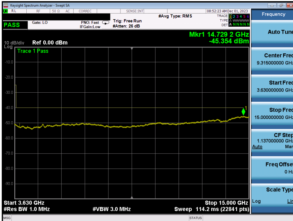
Plot 7-71. Conducted Spurious Plot (ULCA LTE Band 48 - 20+20MHz QPSK - Low Channel)
