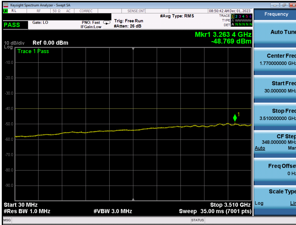
Plot 7-70. Conducted Spurious Plot (ULCA LTE Band 48 - 20+20MHz QPSK - Low Channel)
