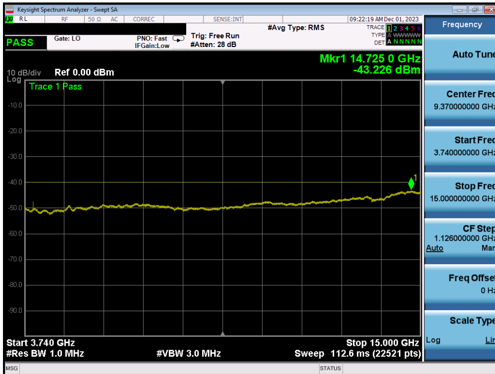
Plot 7-79. Conducted Spurious Plot (ULCA LTE Band 48 - 20+20MHz QPSK - High Channel)
