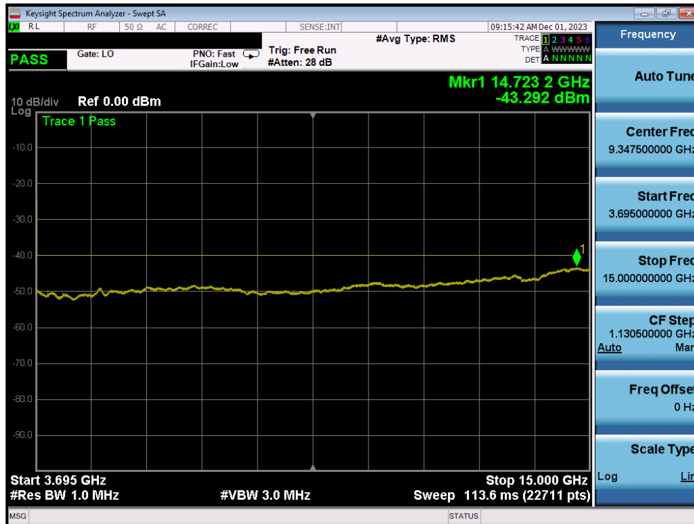
Plot 7-75. Conducted Spurious Plot (ULCA LTE Band 48 - 20+20MHz QPSK - Mid Channel)
