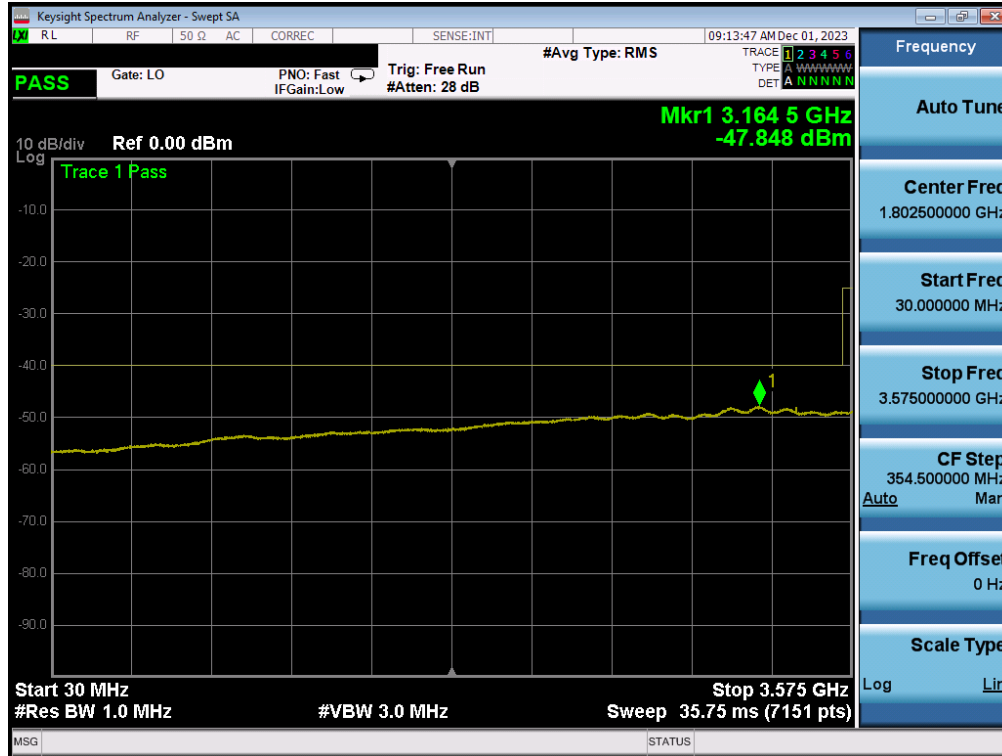
Plot 7-74. Conducted Spurious Plot (ULCA LTE Band 48 - 20+20MHz QPSK - Mid Channel)
