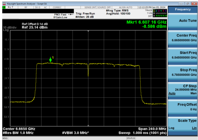
Plot 7-618. Power Spectral Density Plot SDM Diversity Antenna 1b Low Power Indoor (160MHz 802.11ax (UNII Band 7) - Ch. 143, MCS2)
