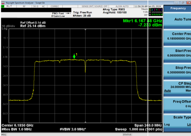
Plot 7-602. Power Spectral Density Plot SDM Diversity Antenna 1b Low Power Indoor (160MHz 802.11ax (UNII Band 5) – Ch. 47, MCS2)
