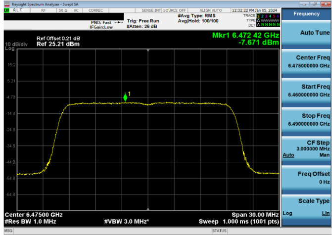
Plot 7-636. Power Spectral Density Plot SDM Diversity Antenna 1b Low Power Indoor (20MHz 802.11ax (UNII Band 6) – Ch. 105, MCS4)
