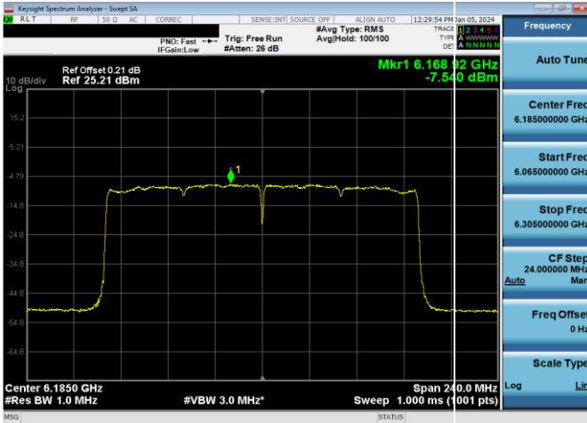
Plot 7-634. Power Spectral Density Plot SDM Diversity Antenna 1b Low Power Indoor (160MHz 802.11ax (UNII Band 5) – Ch. 47, MCS4)
