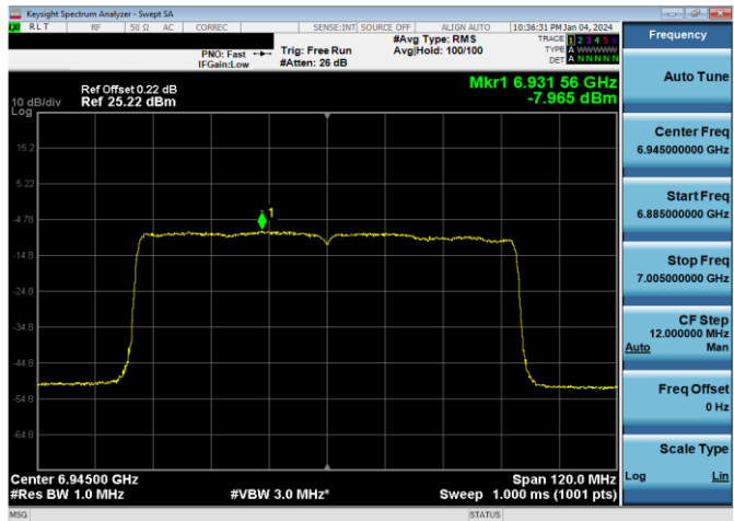
Plot 7-512. Power Spectral Density Plot SDM Primary Antenna 3a Low Power Indoor (80MHz 802.11ax (UNII Band 8) - Ch. 199, MCS4)
