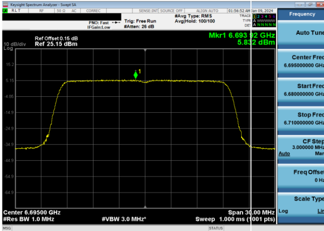
Plot 7-427. Power Spectral Density Plot Antenna 1b Standard Power (20MHz 802.11ax (UNII Band 7) – Ch. 149, MCS2)
