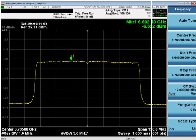
Plot 7-374. Power Spectral Density Plot Antenna 1b Low Power Indoor (80MHz 802.11ax (UNII Band 7) – Ch. 151, MCS2)
