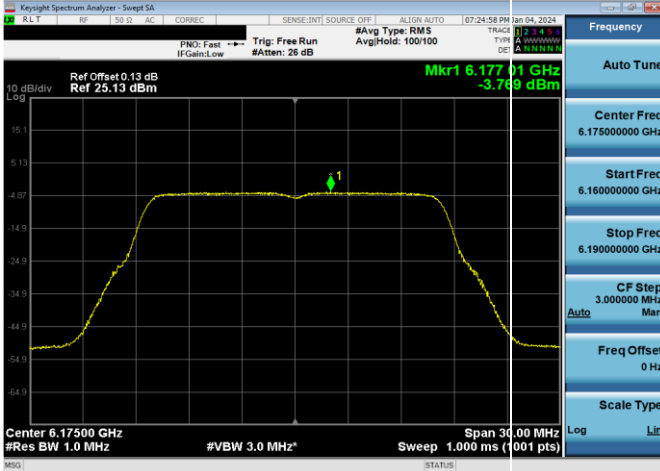
Plot 7-271. Power Spectral Density Plot Antenna 3a Low Power Indoor (20MHz 802.11a (UNII Band 5) – Ch. 45, 12Mbps)
