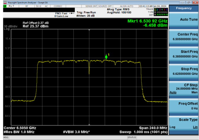
Plot 7-226. Power Spectral Density Plot Antenna 3c Low Power Indoor (160MHz 802.11ax (UNII Band 6) – Ch. 111, MCS11)
