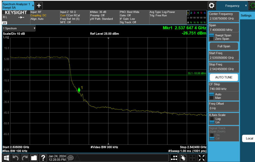
Plot 7-471. Middle Band Edge Plot (NR Band n7 - 5MHz DFT-s-OFDM QPSK – Full RB)
