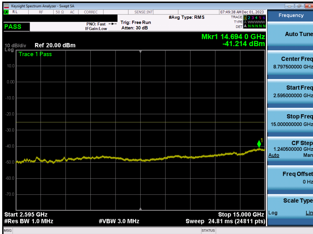
Plot 7-215. Conducted Spurious Plot (ULCA LTE 7 – (20+20)MHz QPSK – RB Size 1, RB Offset 0 – High Channel)
