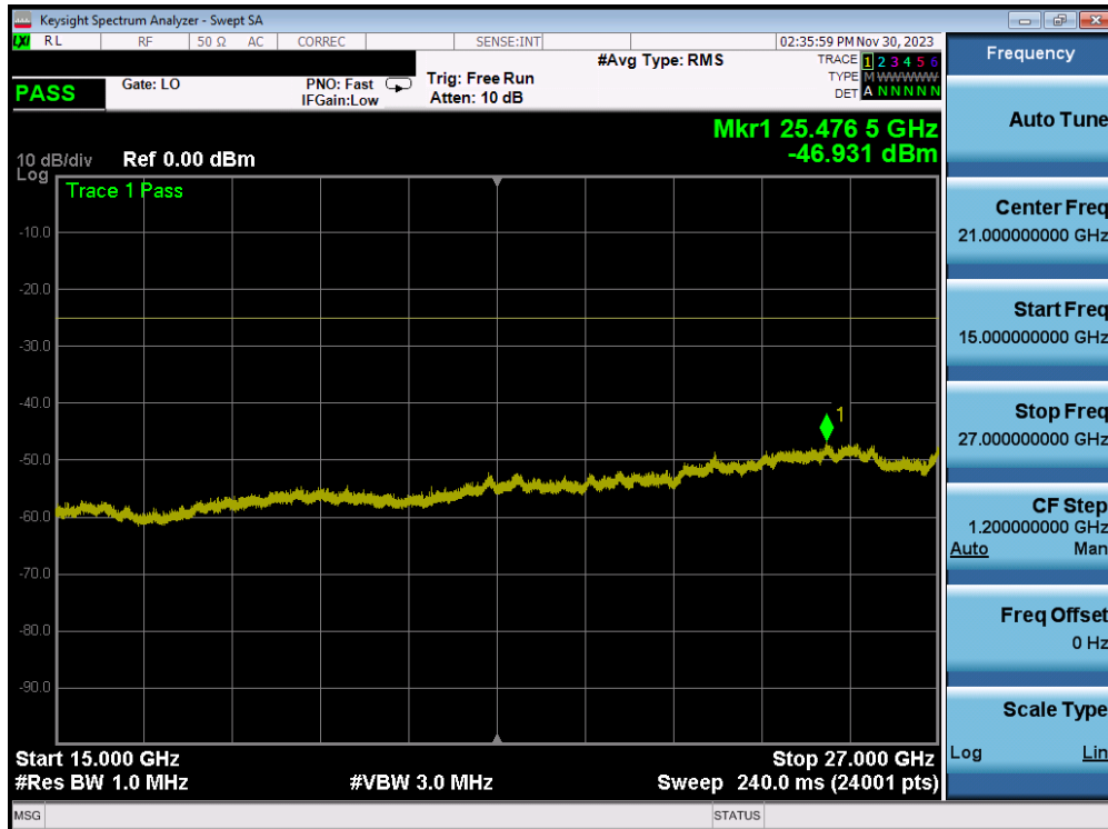
Plot 7-225. Conducted Spurious Plot (ULCA LTE 41 – (20+20)MHz QPSK – RB Size 1, RB Offset 0 – High Channel)
