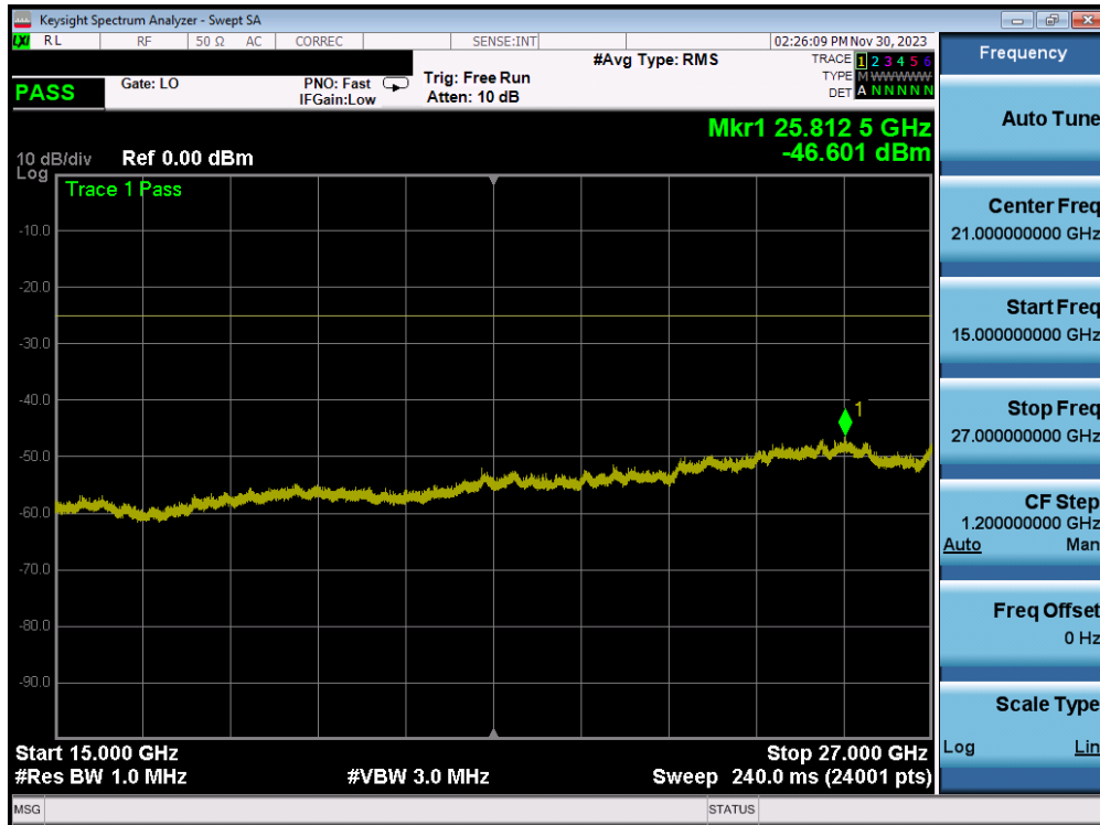
Plot 7-219. Conducted Spurious Plot (ULCA LTE 41 – (20+20)MHz QPSK – RB Size 1, RB Offset 0 – Low Channel)
