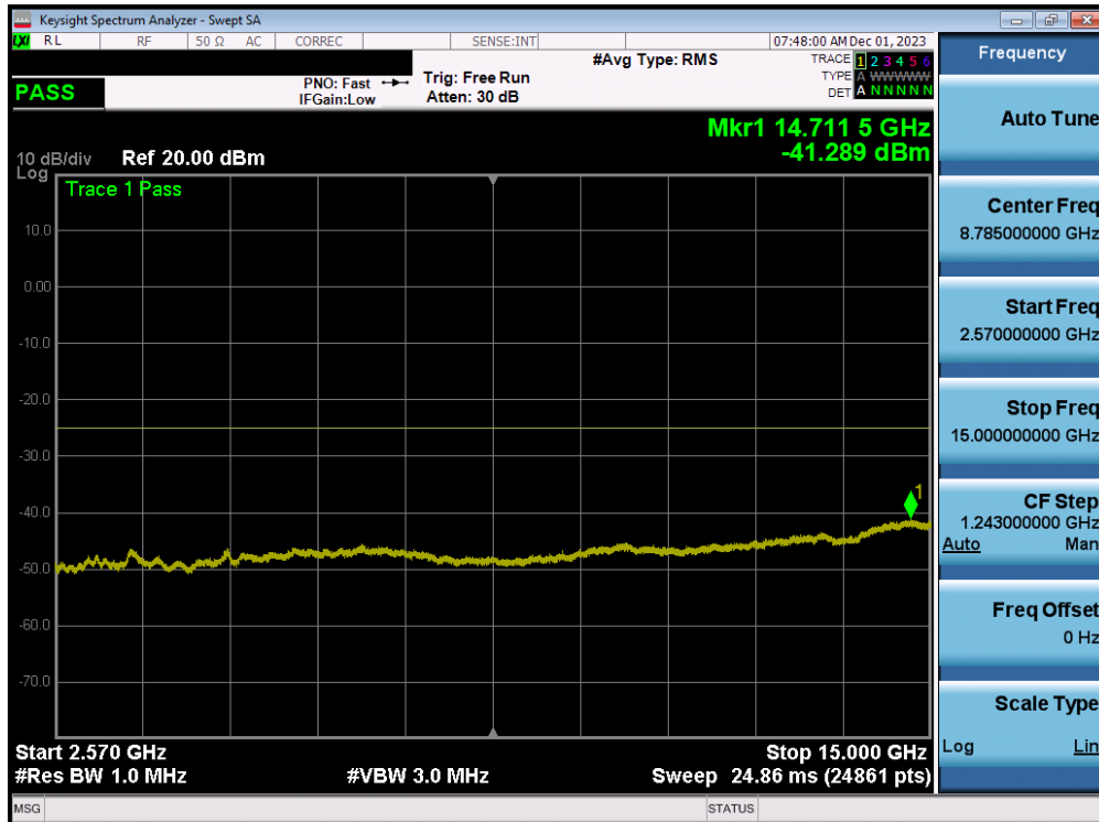
Plot 7-212. Conducted Spurious Plot (ULCA LTE 7 – (20+20)MHz QPSK – RB Size 1, RB Offset 0 – Mid Channel)
