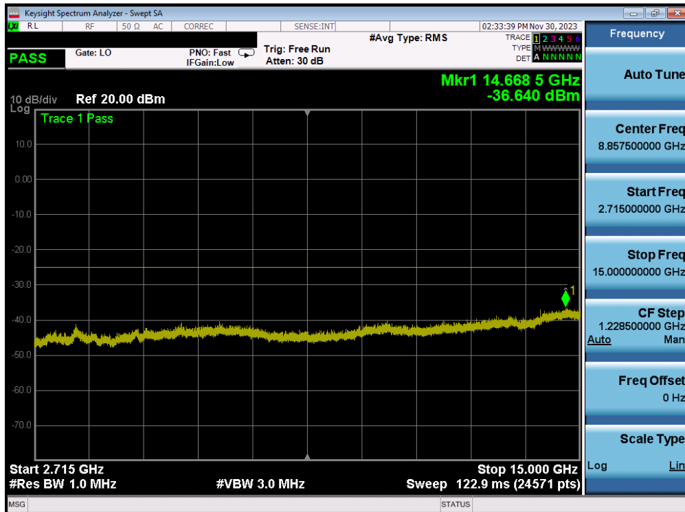
Plot 7-224. Conducted Spurious Plot (ULCA LTE 41 – (20+20)MHz QPSK – RB Size 1, RB Offset 0 – High Channel)
