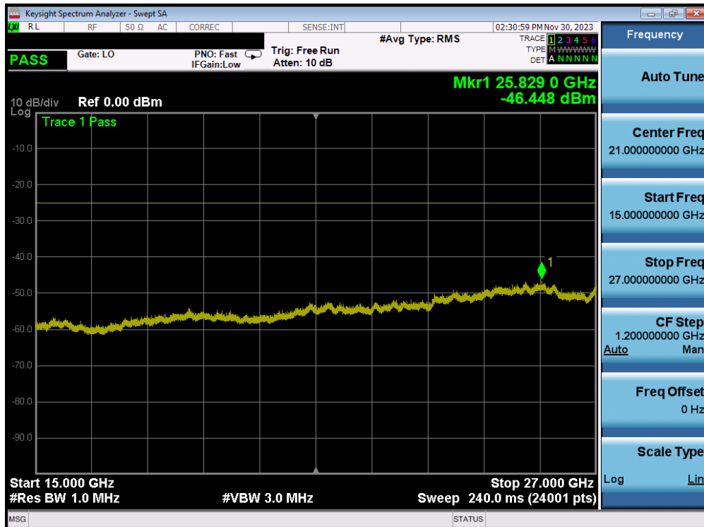
Plot 7-222. Conducted Spurious Plot (ULCA LTE 41 – (20+20)MHz QPSK – RB Size 1, RB Offset 0 – Mid Channel)
