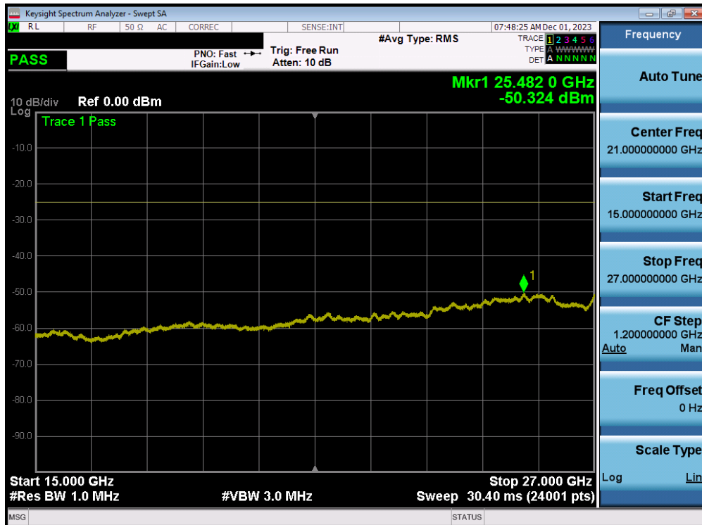
Plot 7-213. Conducted Spurious Plot (ULCA LTE 7 – (20+20)MHz QPSK – RB Size 1, RB Offset 0 – Mid Channel)
