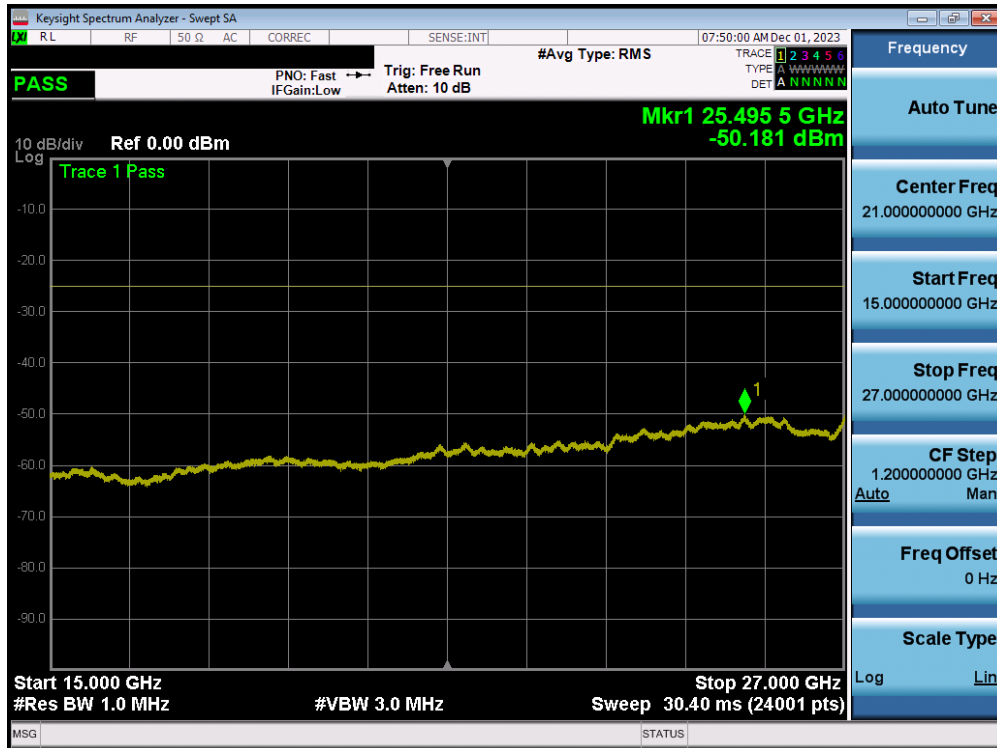
Plot 7-216. Conducted Spurious Plot (ULCA LTE 7 – (20+20)MHz QPSK – RB Size 1, RB Offset 0 – High Channel)
