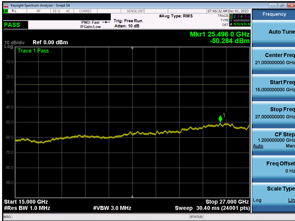
Plot 7-210. Conducted Spurious Plot (ULCA LTE 7 – (20+20)MHz QPSK – RB Size 1, RB Offset 0 – Low Channel)
