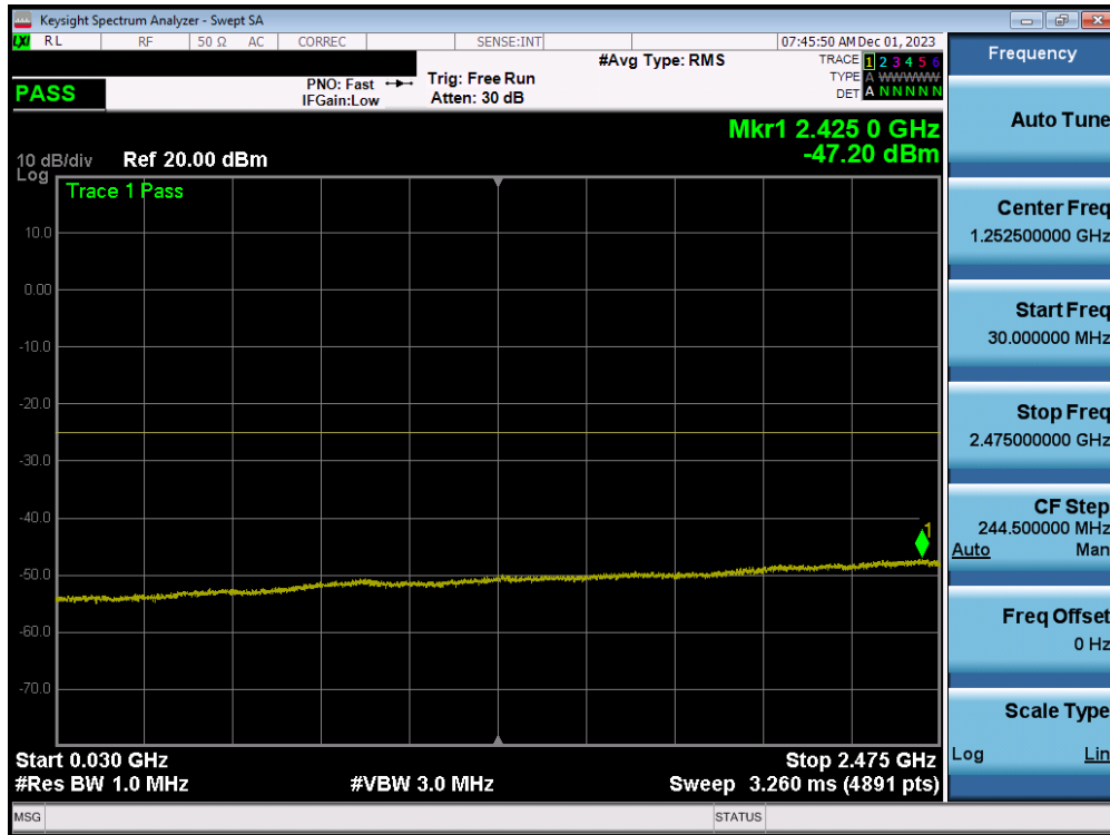
Plot 7-208. Conducted Spurious Plot (ULCA LTE 7 – (20+20)MHz QPSK – RB Size 1, RB Offset 0 – Low Channel)
