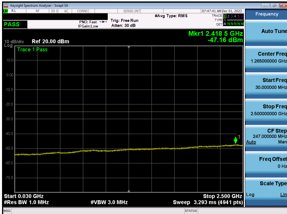
Plot 7-211. Conducted Spurious Plot (ULCA LTE 7 – (20+20)MHz QPSK – RB Size 1, RB Offset 0 – Mid Channel)
