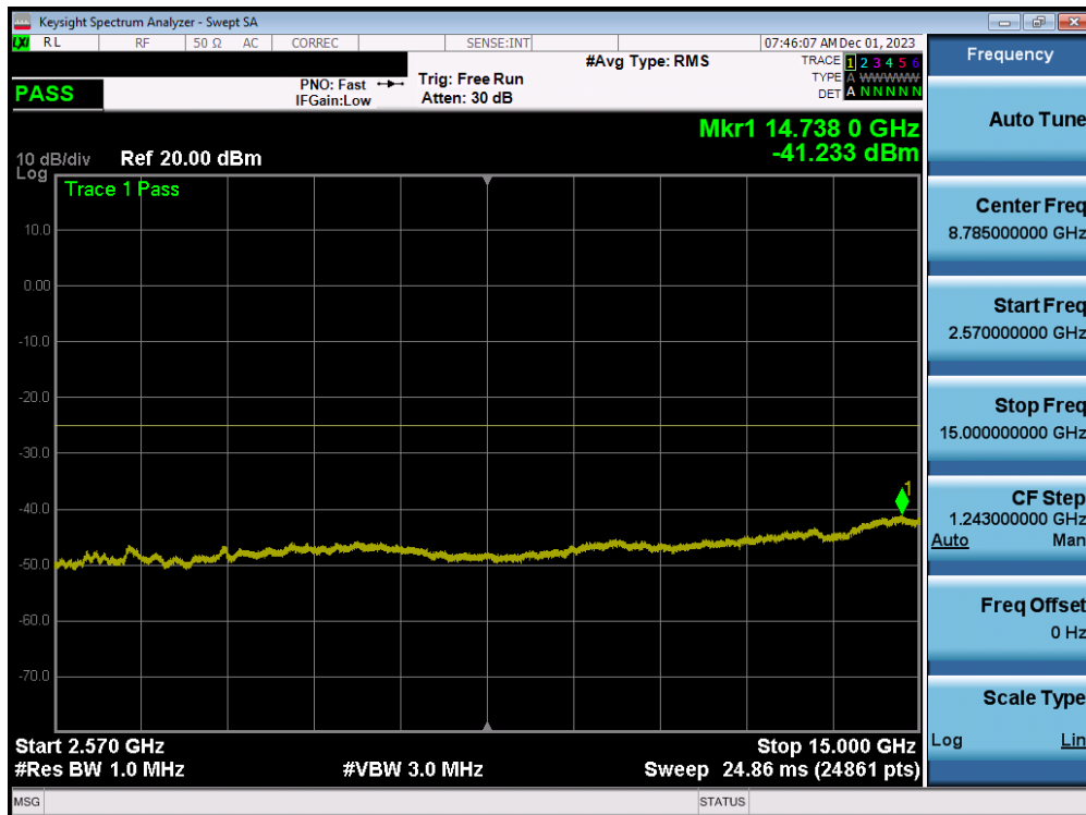
Plot 7-209. Conducted Spurious Plot (ULCA LTE 7 – (20+20)MHz QPSK – RB Size 1, RB Offset 0 – Low Channel)
