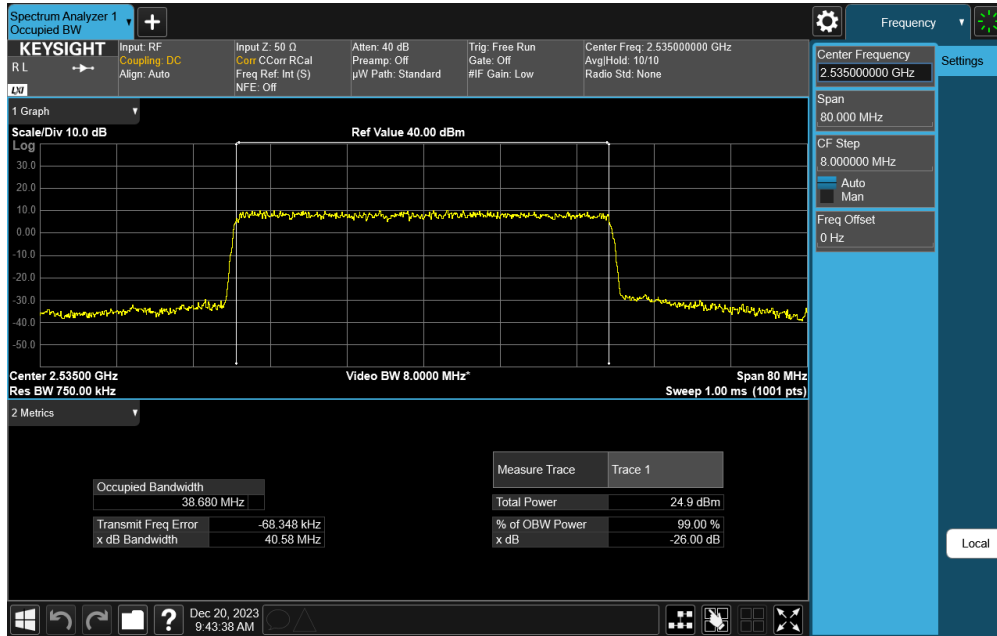
Plot 7-87. Occupied Bandwidth Plot (NR Band n7 - 40MHz DFT-s-OFDM QPSK - Full RB)
