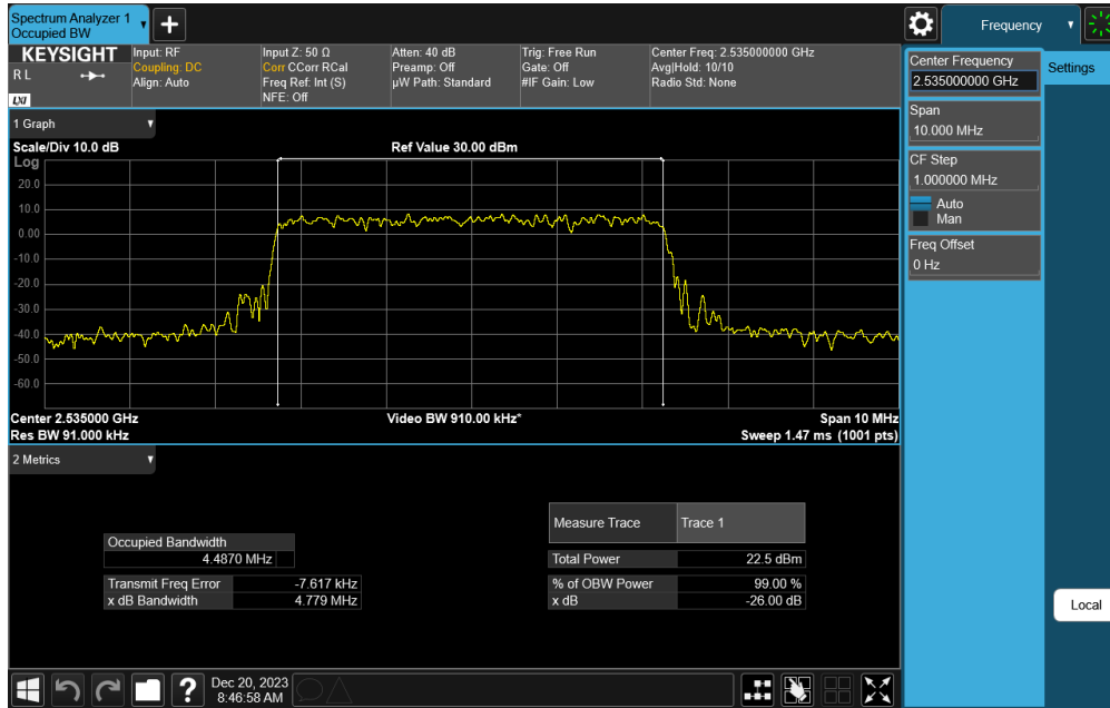
Plot 7-53. Occupied Bandwidth Plot (NR Band n7 - 5MHz CP-OFDM 16-QAM - Full RB)
