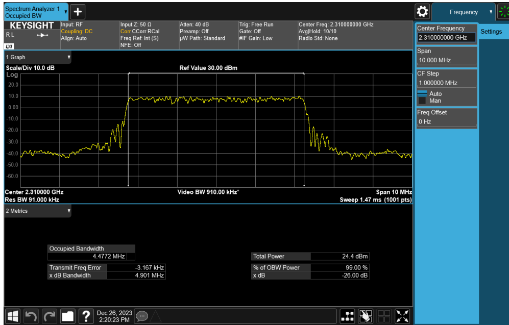
Plot 7-41. Occupied Bandwidth Plot (NR Band n30 - 5MHz DFT-s-OFDM \pi/2 BPSK - Full RB)
