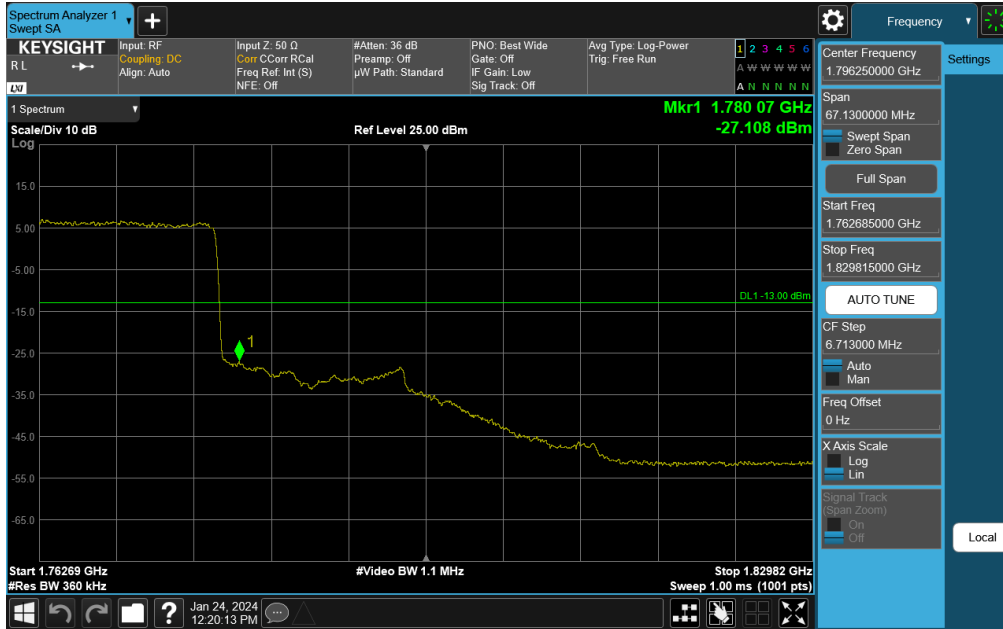
Plot 7-338. Upper Band Edge Plot (NR Band n66 – 35.0MHz DFT-s-OFDM \pi/2 BPSK - Full RB)
