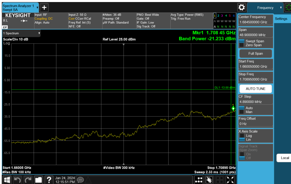
Plot 7-329. Lower Extended Band Edge Plot (NR Band n66 – 25.0MHz DFT-s-OFDM \pi/2 BPSK - Full RB)
