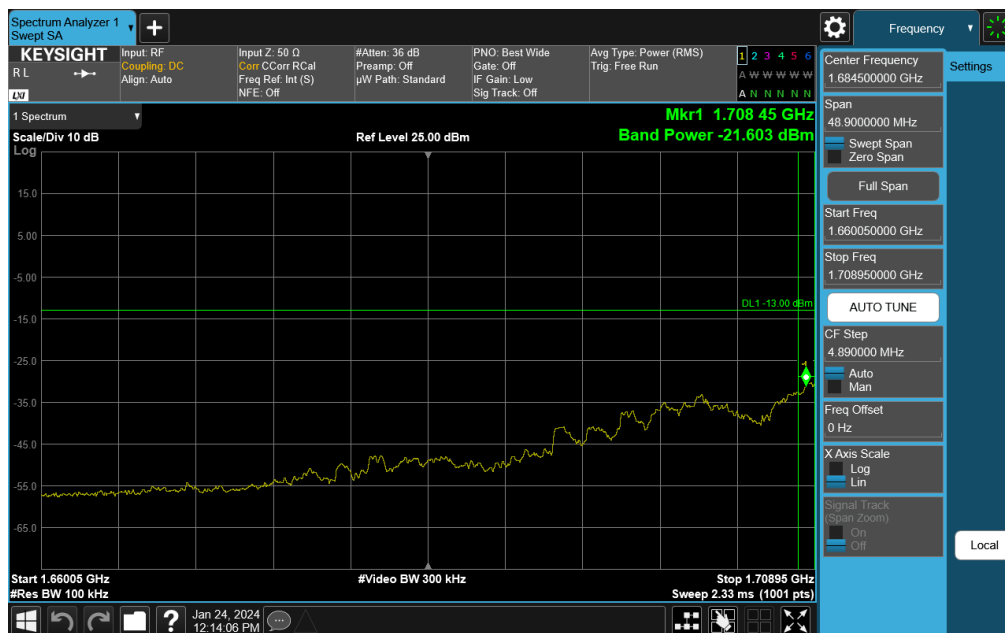
Plot 7-325. Lower Extended Band Edge Plot (NR Band n66 – 20.0MHz DFT-s-OFDM \pi/2 BPSK - Full RB)
