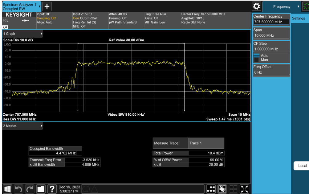
Plot 7-144. Occupied Bandwidth Plot (NR Band n12 - 5MHz CP-OFDM 256-QAM - Full RB)
