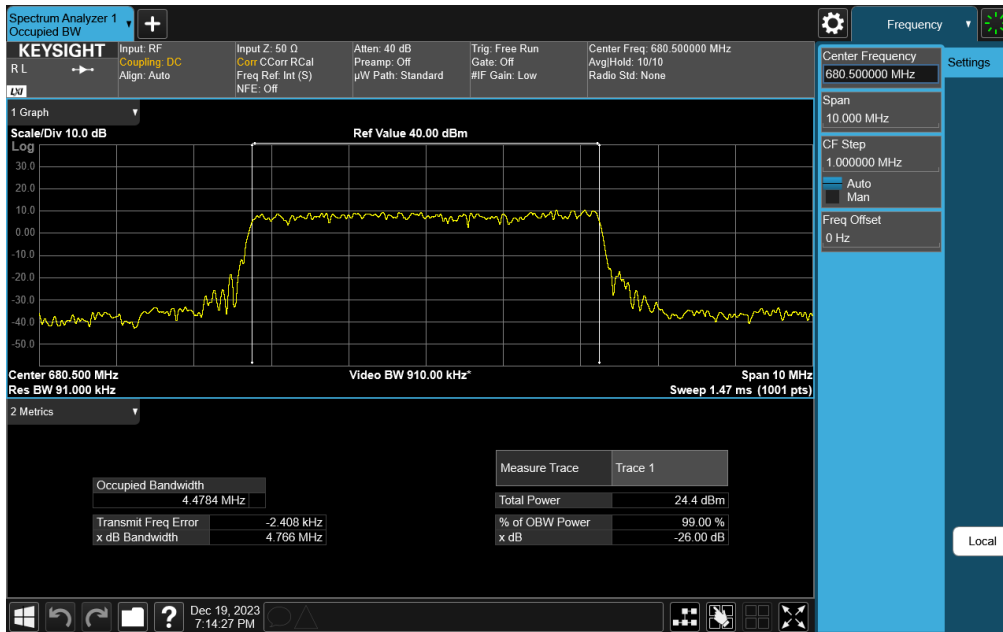
Plot 7-121. Occupied Bandwidth Plot (NR Band n71 - 5MHz DFT-s-OFDM QPSK - Full RB)
