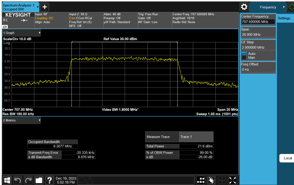
Plot 7-148. Occupied Bandwidth Plot (NR Band n12 - 10MHz CP-OFDM 64-QAM - Full RB)
