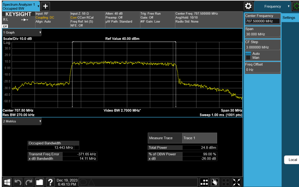
Plot 7-150. Occupied Bandwidth Plot (NR Band n12 - 15MHz DFT-s-OFDM \pi/2 BPSK - Full RB)
