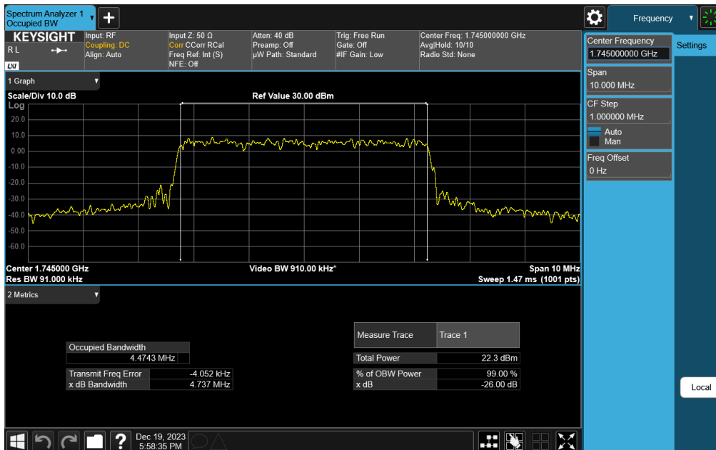
Plot 7-66. Occupied Bandwidth Plot (NR Band n66 - 5.0MHz CP-OFDM QPSK - Full RB)
