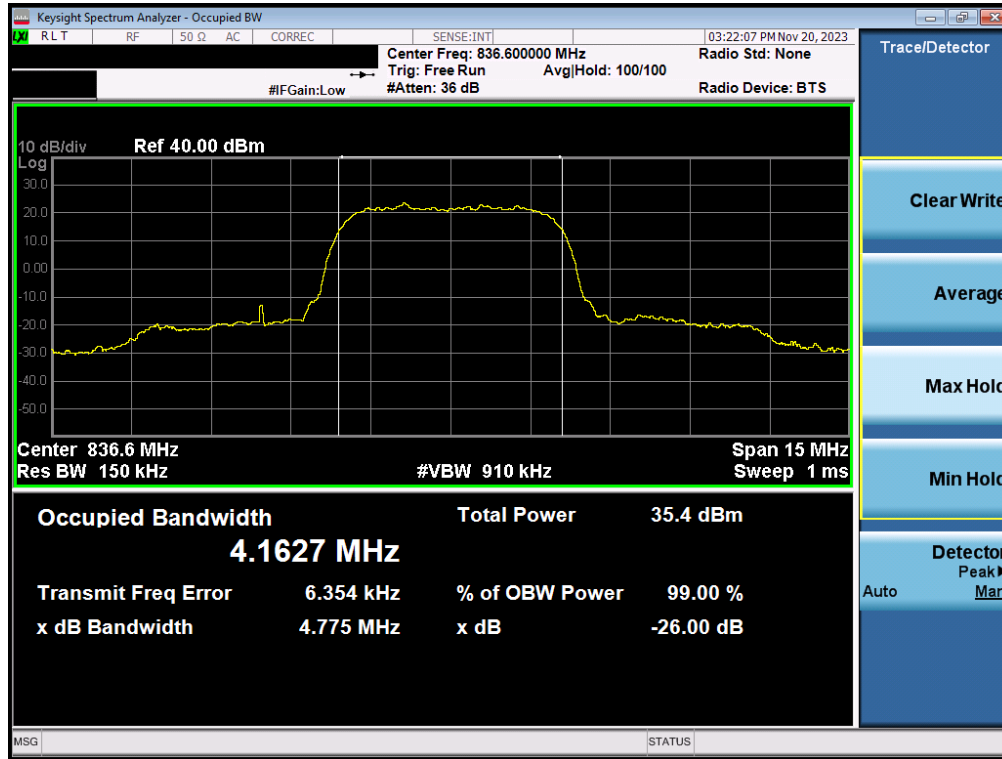
Plot 7-41. Occupied Bandwidth Plot (WCDMA, Ch. 4183)
