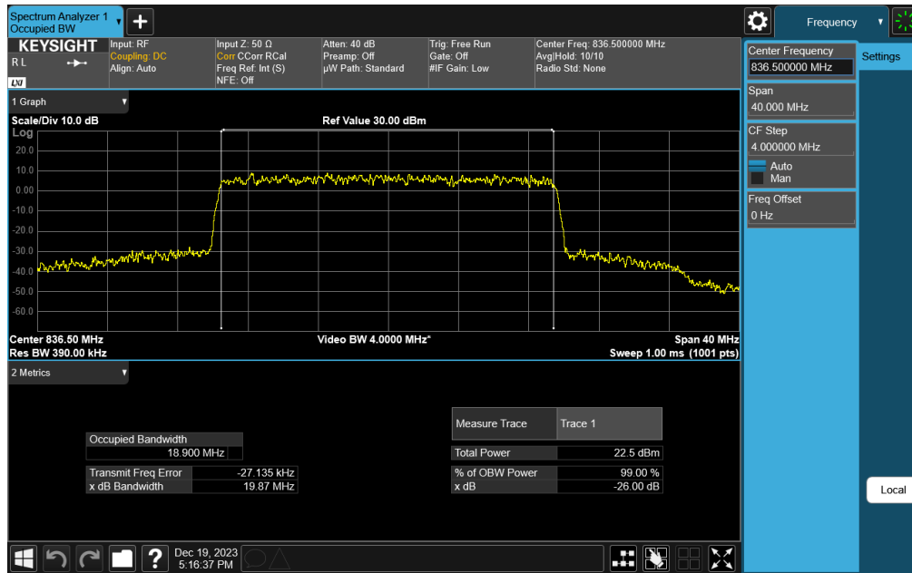
Plot 7-37. Occupied Bandwidth Plot (NR Band n26/n5 - 20MHz CP-OFDM QPSK - Full RB Configuration)
