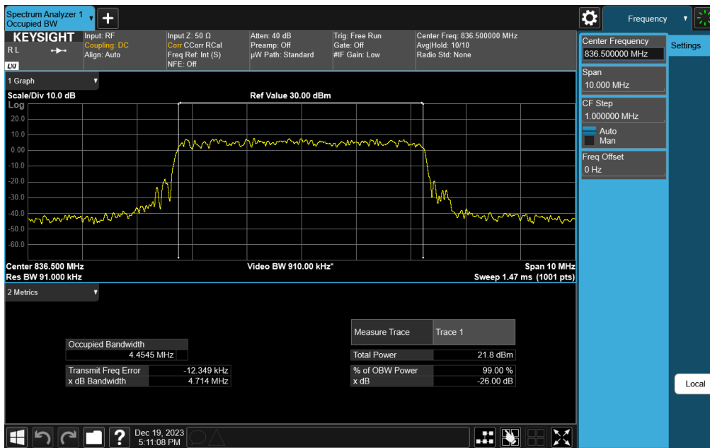
Plot 7-24. Occupied Bandwidth Plot (NR Band n26/n5 - 5MHz CP-OFDM 64-QAM - Full RB Configuration)
