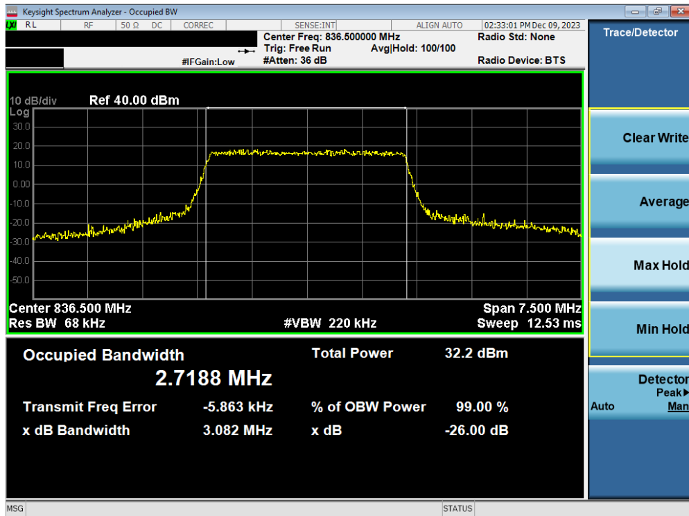
Plot 7-6. Occupied Bandwidth Plot (LTE Band 26/5 - 3MHz 16-QAM - Full RB Configuration)
