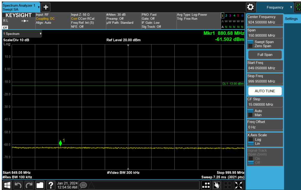
Plot 7-61. Conducted Spurious Plot (NR Band n26/n5 - 20.0MHz DFT-s-OFDM QPSK - RB Size 1, RB Offset 0 - Low Channel)
