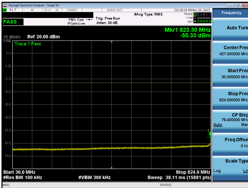
Plot 7-72. Conducted Spurious Plot (WCDMA Ch. 4183)
