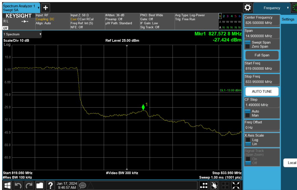
Plot 7-117. Upper Band Edge Plot (NR Band n26 - 10MHz DFT-s-OFDM \pi/2 BPSK – Mid Channel)
