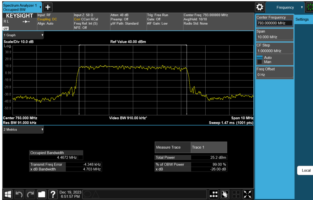
Plot 7-25. Occupied Bandwidth Plot (NR Band 14 - 5MHz DFT-s-OFDM \pi/2 BPSK - Full RB)
