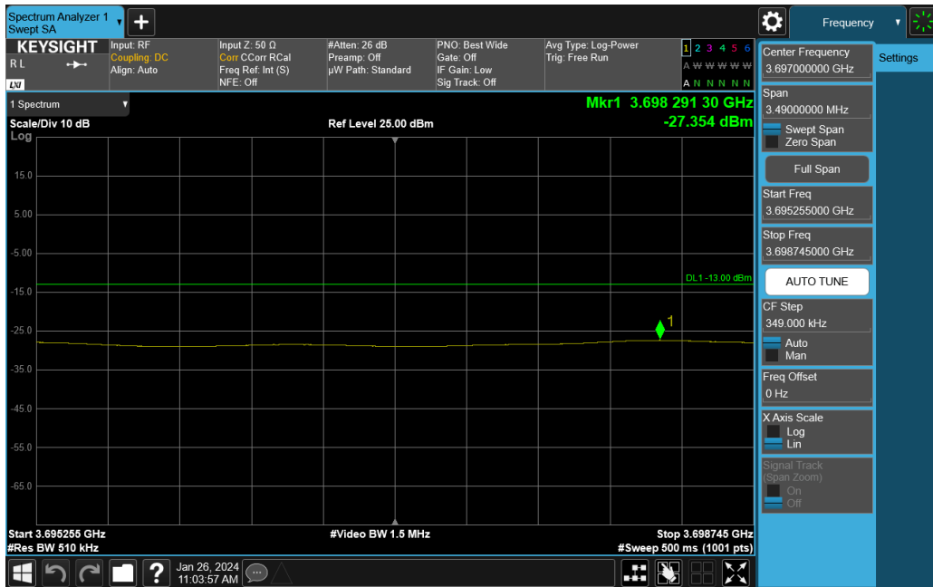
Plot 7-226. Lower ACP Plot (NR Band n77 - 15MHz DFT-s-OFDM QPSK – Full RB)
