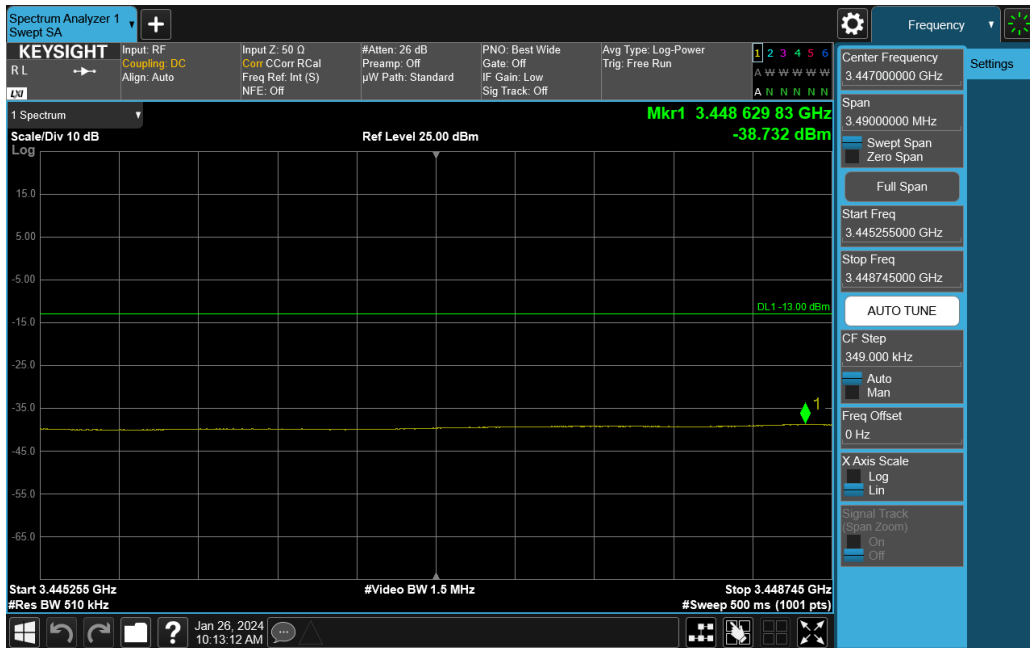
Plot 7-194. Lower ACP Plot (NR Band n77 - 80MHz DFT-s-OFDM QPSK – Full RB)
