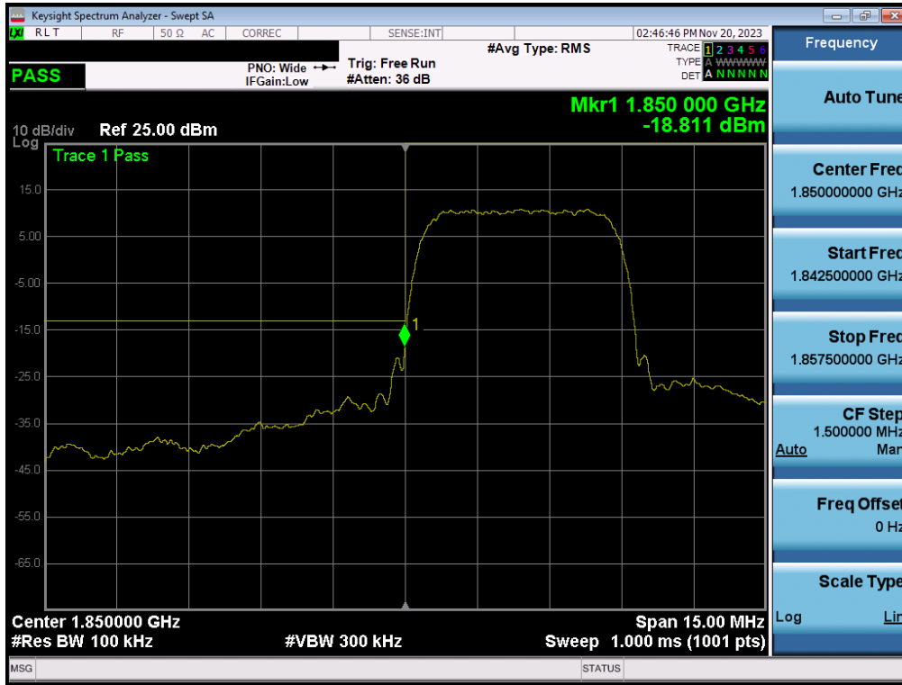
Plot 7-189. Lower Band Edge Plot (WCDMA PCS – Ch. 9262)
