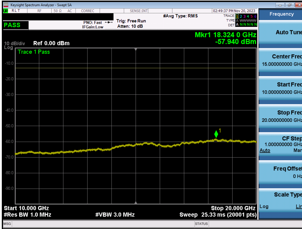
Plot 7-86. Conducted Spurious Plot (WCDMA Ch. 9262)
