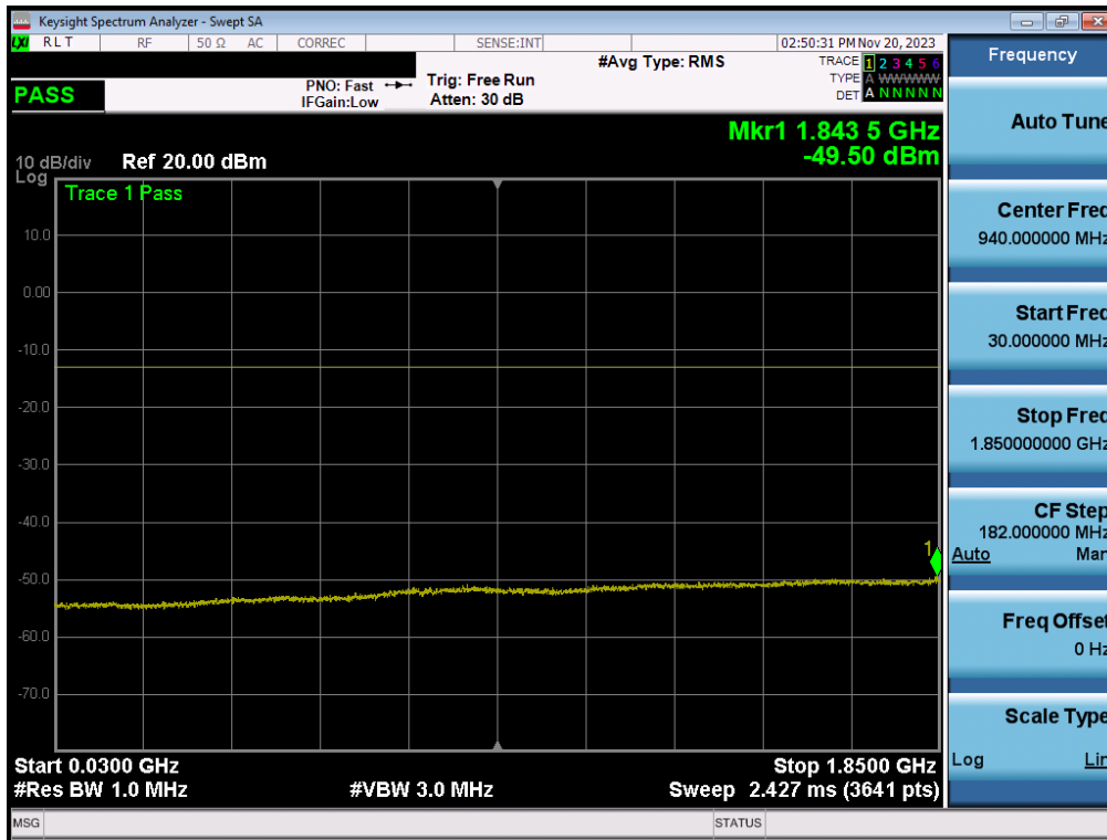
Plot 7-87. Conducted Spurious Plot (WCDMA Ch. 9400)
