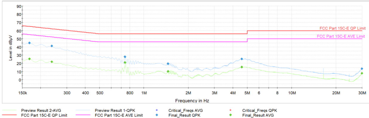
Plot 7-196. AC Line Conducted Emissions with 802.11ax (RU26) Ch.6 CDD (L1, with AC/DC Adapter)
