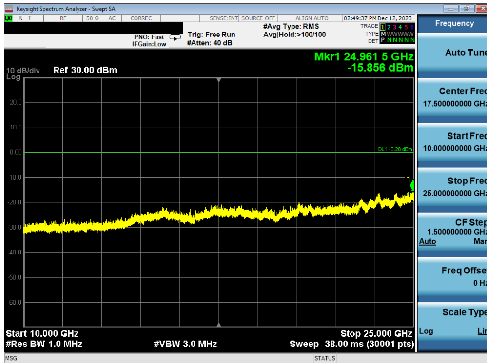
Plot 7-114. Conducted Spurious Plot Antenna WF8 (802.11ax OFDMA – RU242 – Ch. 6)
