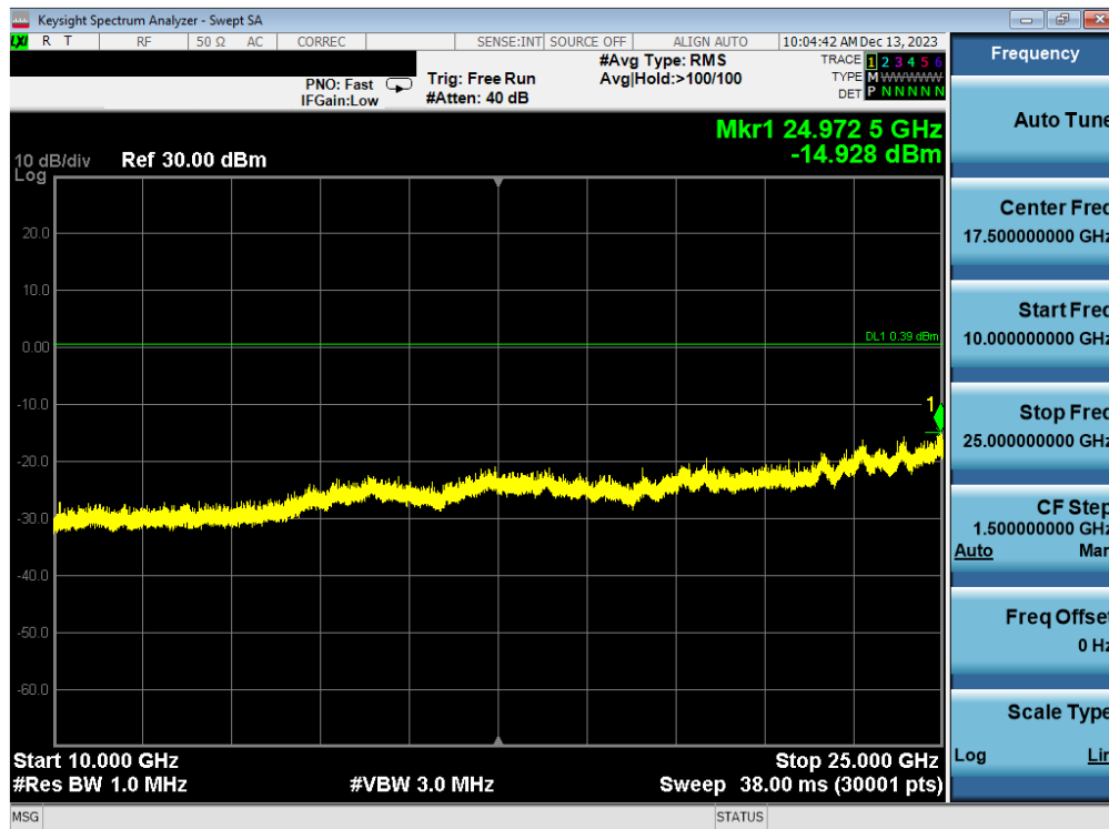
Plot 7-120. Conducted Spurious Plot Antenna WF7b (802.11ax OFDMA – RU26 – Ch. 6)
