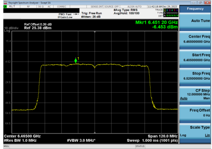
Plot 7-284. LPI Power Spectral Density Plot Antenna WF8 (80MHz 802.11ax RU996 (UNII Band 6) – Ch. 103)
