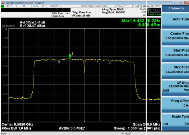
Plot 7-288. LPI Power Spectral Density Plot Antenna WF8 (160MHz 802.11ax RU996x2 (UNII Band 6) – Ch. 111)
