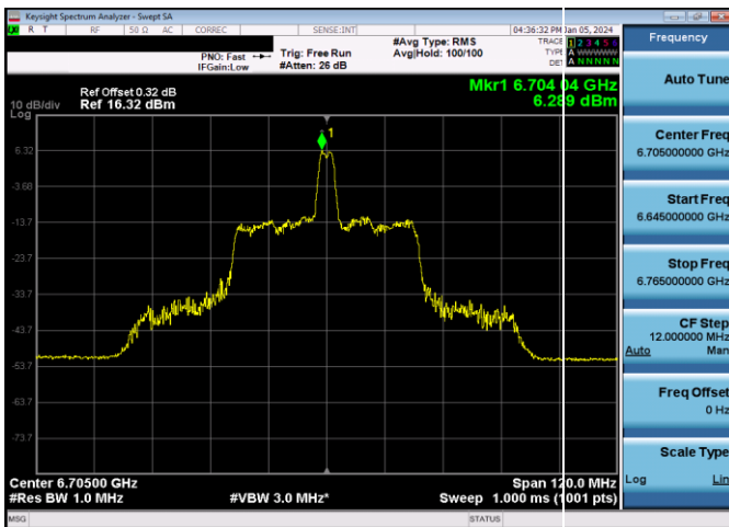
Plot 7-243. SP Power Spectral Density Plot SDM Antenna WF8 (80MHz 802.11ax RU26 (UNII Band 7) – Ch. 151)
