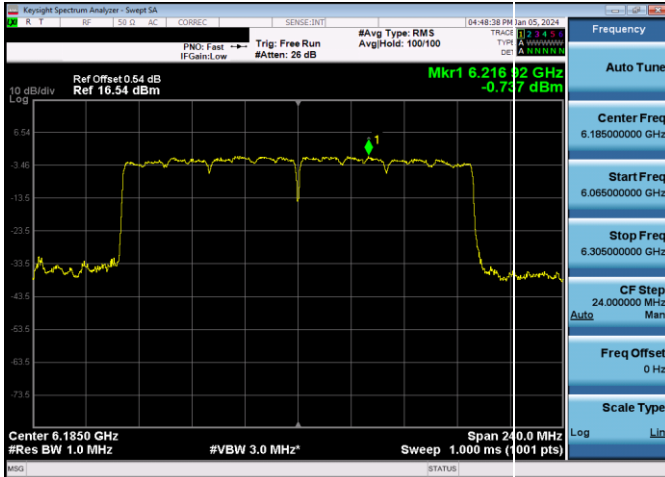
Plot 7-223. SP Power Spectral Density Plot SDM Antenna WF8 (160MHz 802.11ax RU996x2 (UNII Band 5) – Ch. 47)
