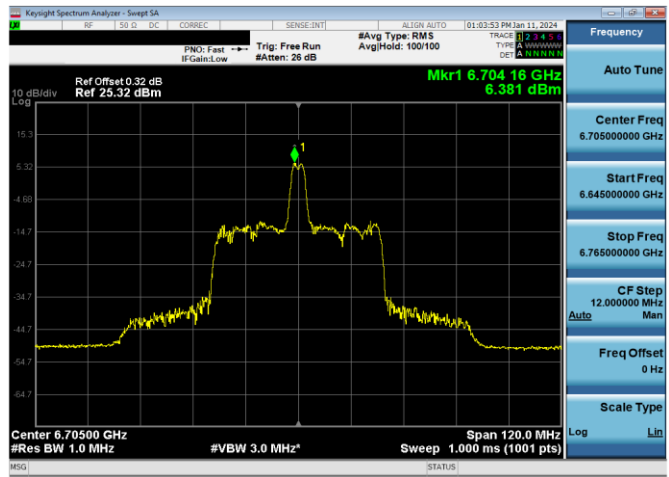
Plot 7-244. SP Power Spectral Density Plot SDM Antenna WF7a (80MHz 802.11ax RU26 (UNII Band 7) – Ch. 151)
