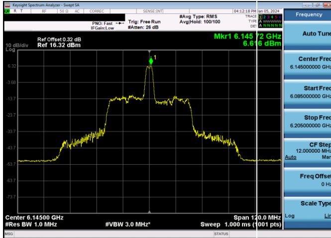
Plot 7-211. SP Power Spectral Density Plot SDM Antenna WF8 (80MHz 802.11ax RU26 (UNII Band 5) – Ch. 39)
