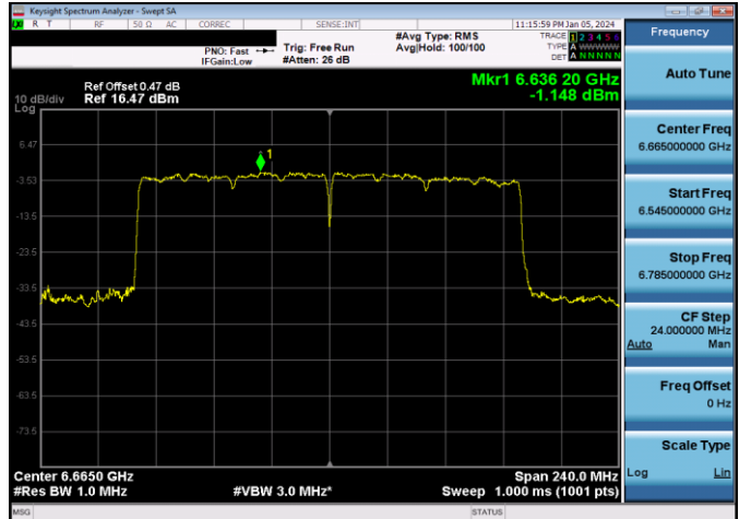
Plot 7-192. SP Power Spectral Density Plot Antenna WF7a (160MHz 802.11ax RU996x2 (UNII Band 7) – Ch. 143)
