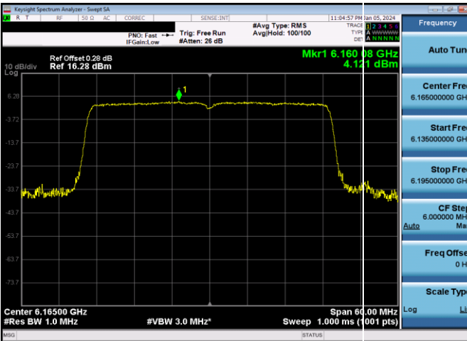
Plot 7-168. SP Power Spectral Density Plot Antenna WF7a (40MHz 802.11ax RU484 (UNII Band 5) – Ch. 43)
