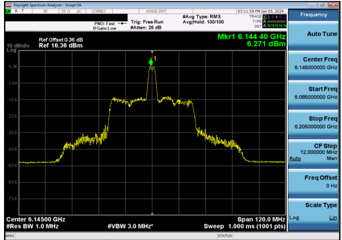
Plot 7-138. SP Power Spectral Density Plot Antenna WF8 (80MHz 802.11ax RU26 (UNII Band 5) – Ch. 39)
