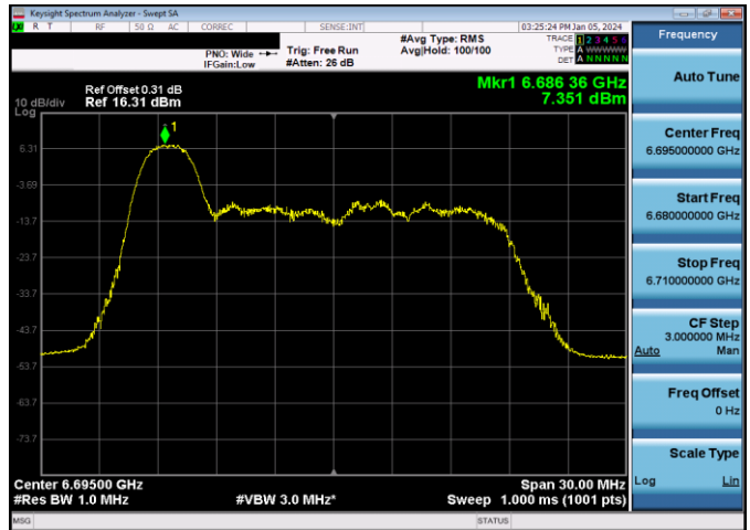
Plot 7-145. SP Power Spectral Density Plot Antenna WF8 (20MHz 802.11ax RU26 (UNII Band 7) – Ch. 149)
