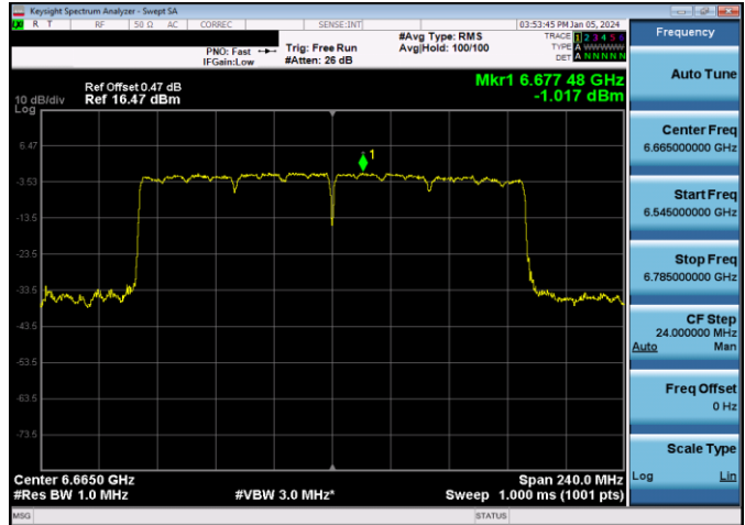
Plot 7-160. SP Power Spectral Density Plot Antenna WF8 (160MHz 802.11ax RU996x2 (UNII Band 7) – Ch. 143)
