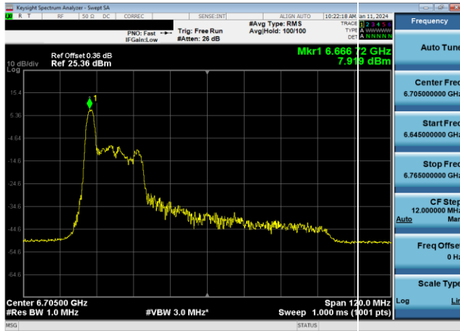
Plot 7-185. SP Power Spectral Density Plot Antenna WF7a (80MHz 802.11ax RU26 (UNII Band 7) – Ch. 151)
