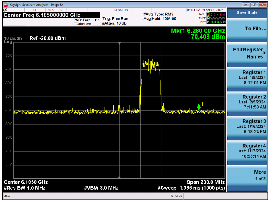
Plot 7-804. 160MHz Bandwidth – AWGN Signal Injected at High End – Channel 47
