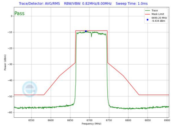
Plot 7-646. In-Band Emission Plot SDM Antenna WF7a Low Power Indoor (80MHz 802.11ax (UNII Band 7) – Ch. 151, MCS2)
