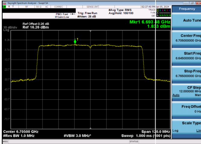
Plot 7-425. Power Spectral Density Plot SDM Antenna WF8 Standard Power (80MHz 802.11ax (UNII Band 7) – Ch. 151, MCS4)
