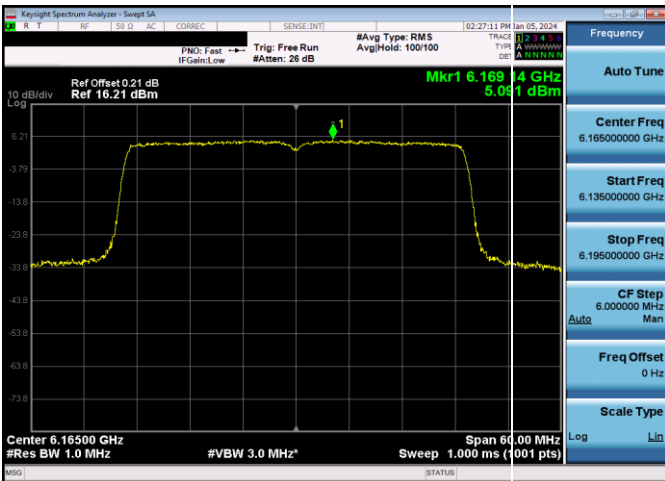
Plot 7-415. Power Spectral Density Plot SDM Antenna WF8 Standard Power (40MHz 802.11ax (UNII Band 5) – Ch. 43, MCS4)
