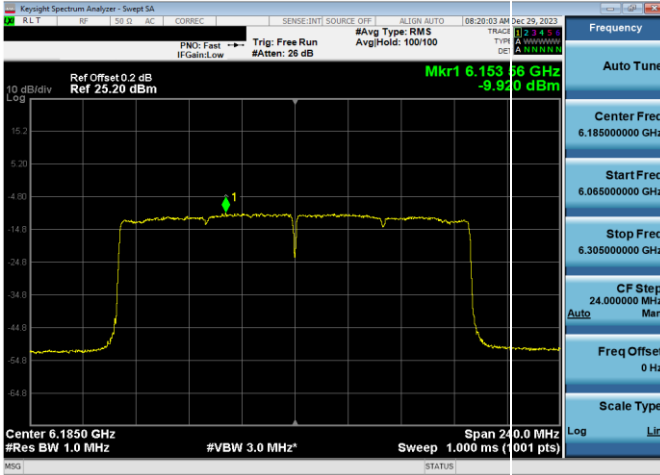
Plot 7-307. Power Spectral Density Plot SDM Antenna WF8 Low Power Indoor (160MHz 802.11ax (UNII Band 5) – Ch. 47, MCS2)
