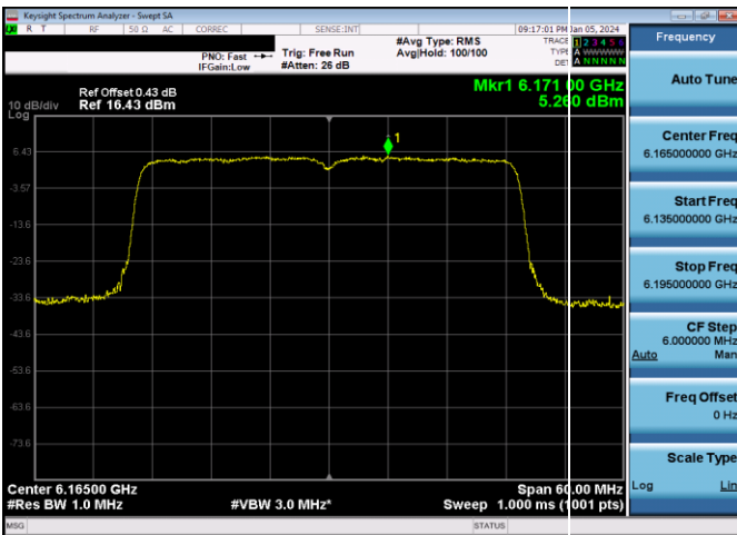
Plot 7-293. Power Spectral Density Plot Antenna WF7a Standard Power (40MHz 802.11ax (UNII Band 5) - Ch. 43, MCS11)
