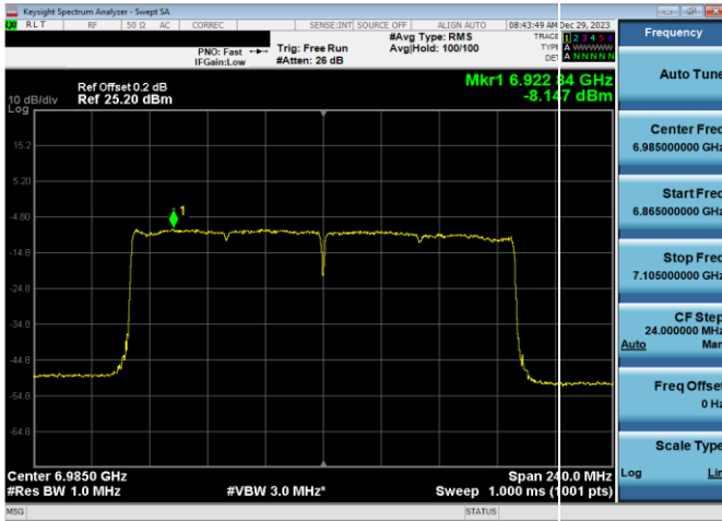
Plot 7-331. Power Spectral Density Plot SDM Antenna WF8 Low Power Indoor (160MHz 802.11ax (UNII Band 8) – Ch. 207, MCS2)
