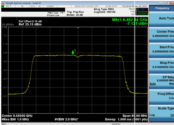
Plot 7-218. Power Spectral Density Plot Antenna WF7a Low Power Indoor (40MHz 802.11ax (UNII Band 6) - Ch. 107, MCS2)
