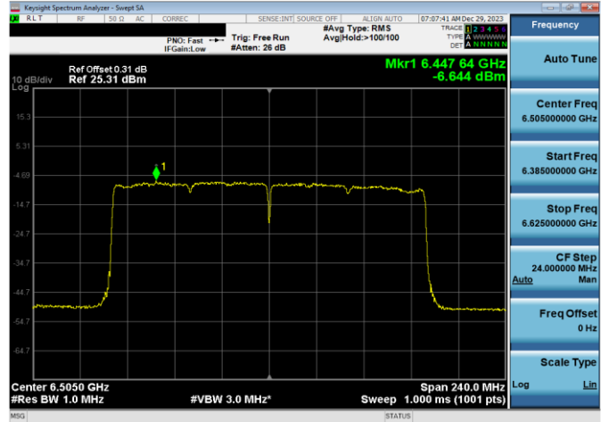
Plot 7-150. Power Spectral Density Plot Antenna WF8 Low Power Indoor (160MHz 802.11ax (UNII Band 6) - Ch. 111, MCS4)
