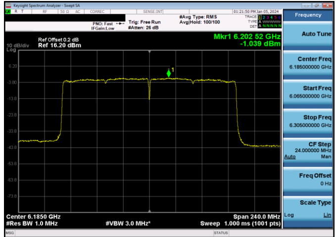
Plot 7-185. Power Spectral Density Plot Antenna WF8 Standard Power (160MHz 802.11ax (UNII Band 5) – Ch. 47, MCS2)
