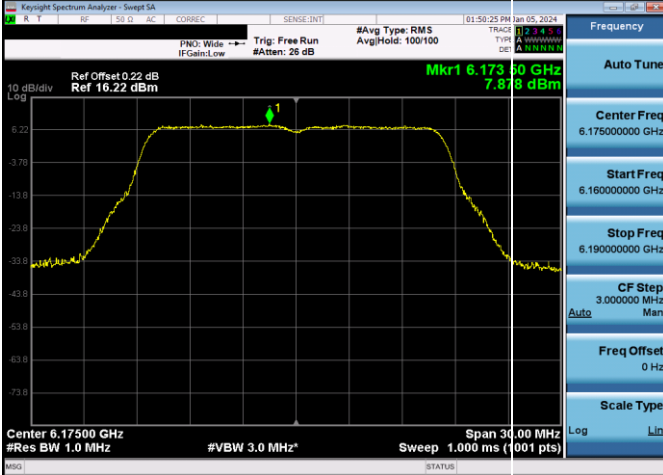
Plot 7-201. Power Spectral Density Plot Antenna WF8 Standard Power (20MHz 802.11a (UNII Band 5) – Ch. 45, 54Mbps)
