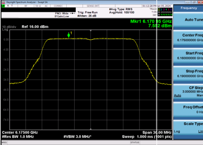
Plot 7-181. Power Spectral Density Plot Antenna WF8 Standard Power (20MHz 802.11a (UNII Band 5) – Ch. 45, 12Mbps)
