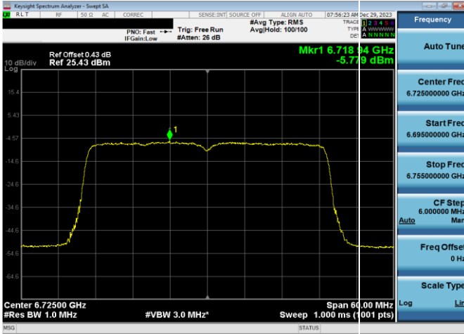
Plot 7-169. Power Spectral Density Plot Antenna WF8 Low Power Indoor (40MHz 802.11ax (UNII Band 7) – Ch. 155, MCS11)
