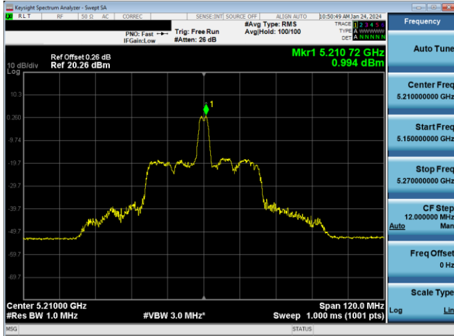
Plot 7-385. ISED PSD SDM Antenna WF8 (80MHz BW 11ax Index 18 - RU26 - Ch.42)
