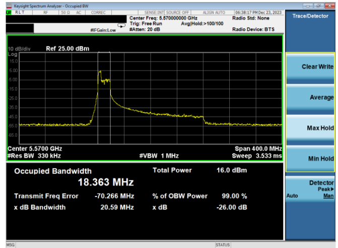
Plot 7-85. 26dB BW & 99% OBW Antenna WF7a (160MHz BW 11ax Index 37 – RU52 – Ch.114 (L))
