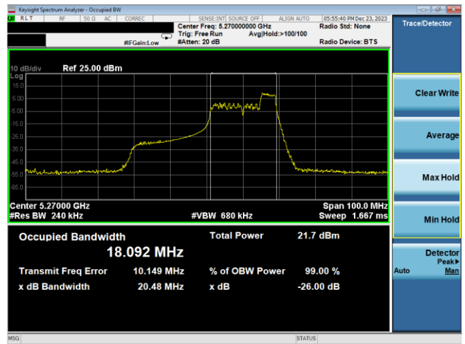
Plot 7-67. 26dB BW & 99% OBW Antenna WF7a (40MHz BW 11ax Index 44 – RU52 – Ch.54)
