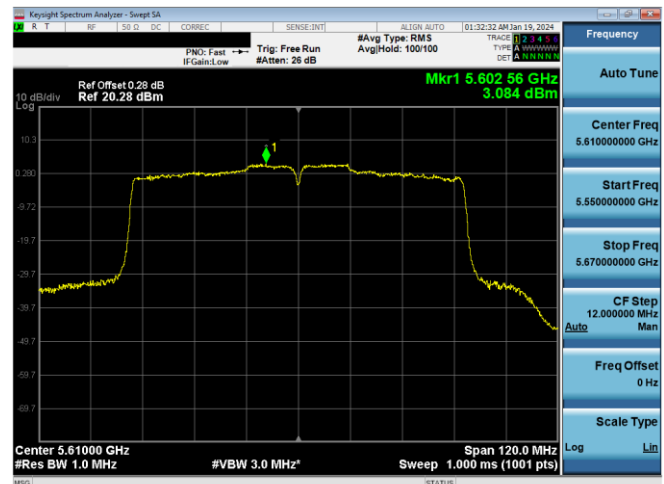
Plot 7-306. PSD Antenna WF7a (80MHz BW 802.11ac – Ch. 122, MCS4)
