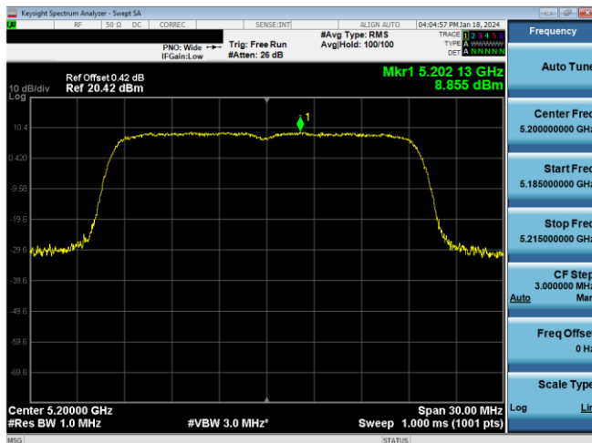
Plot 7-209. PSD Antenna WF8 (20MHz BW 802.11ax(SU) – Ch. 40, MCS11)
