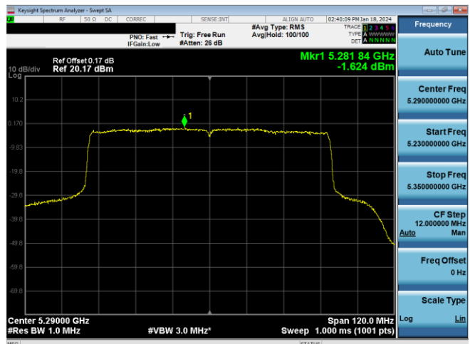
Plot 7-179. PSD Antenna WF8 (80MHz BW 802.11ax(SU) – Ch. 58, MCS2)
