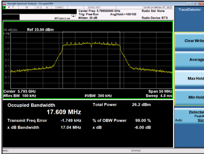
Plot 7-132. 6dB BW & 99% OBW Antenna WF8 (20MHz BW 802.11n – Ch. 157, MCS2)
