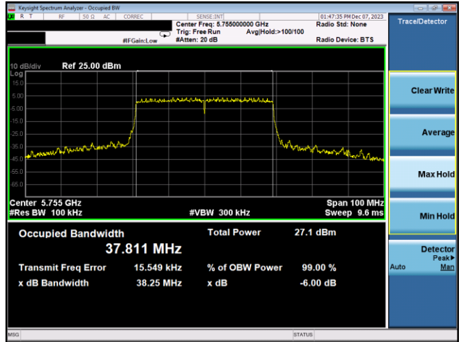
Plot 7-147. 6dB BW & 99% OBW Antenna WF8 (40MHz BW 802.11ax(SU) - Ch. 151, MCS11)
