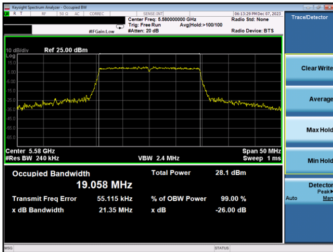
Plot 7-125. 26dB BW & 99% OBW Antenna WF7a (20MHz BW 802.11ax(SU) – Ch. 116, MCS11)
