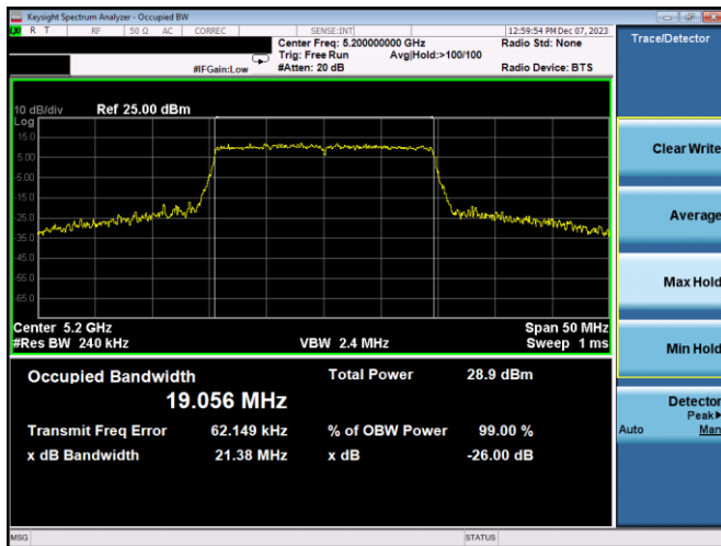
Plot 7-46. 26dB BW & 99% OBW Antenna WF8 (20MHz BW 802.11ax(SU) – Ch. 40, MCS11)
