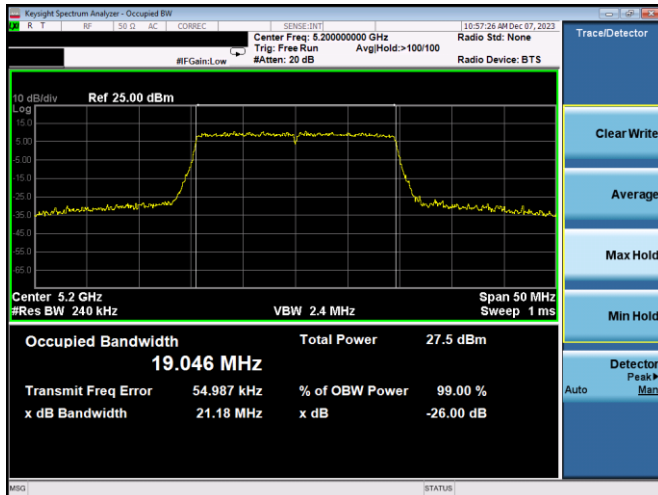
Plot 7-24. 26dB BW & 99% OBW Antenna WF8 (20MHz BW 802.11ax(SU) – Ch. 40, MCS4)
