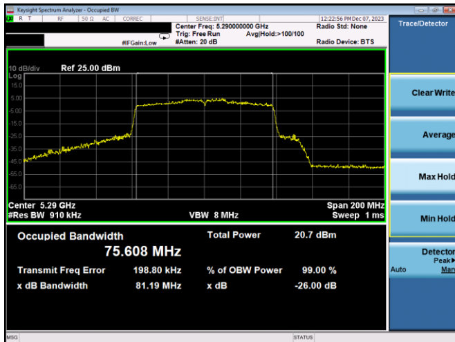
Plot 7-35. 26dB BW & 99% OBW Antenna WF8 (80MHz BW 802.11ac – Ch. 58, MCS4)
