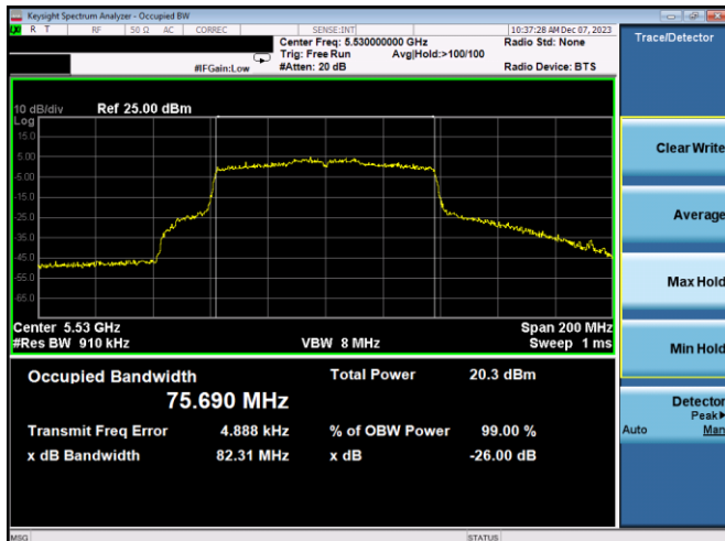
Plot 7-19. 26dB BW & 99% OBW Antenna WF8 (80MHz BW 802.11ac – Ch. 106, MCS2)
