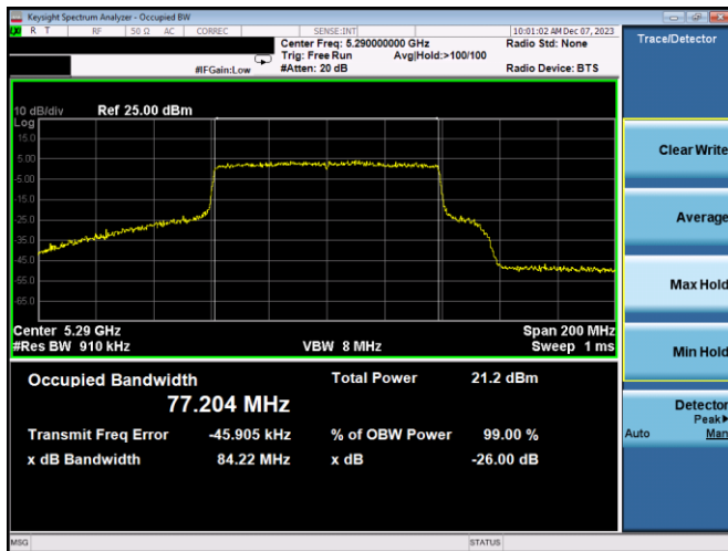
Plot 7-14. 26dB BW & 99% OBW Antenna WF8 (80MHz BW 802.11ax(SU) – Ch. 58, MCS2)
