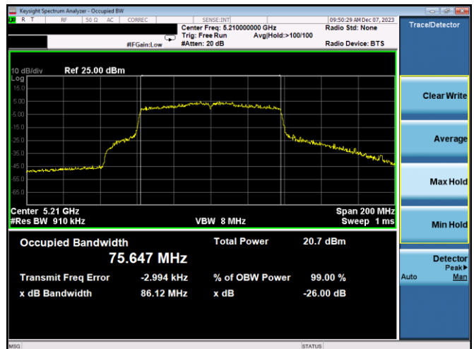
Plot 7-5. 26dB BW & 99% OBW Antenna WF8 (80MHz BW 802.11ac – Ch. 42, MCS2)
