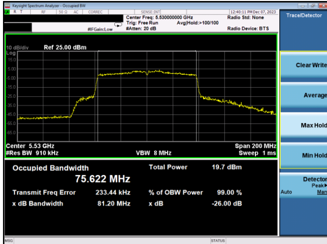
Plot 7-41. 26dB BW & 99% OBW Antenna WF8 (80MHz BW 802.11ac – Ch. 106, MCS4)
