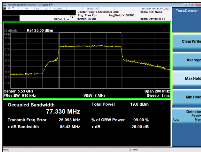
Plot 7-20. 26dB BW & 99% OBW Antenna WF8 (80MHz BW 802.11ax(SU) – Ch. 106, MCS2)
