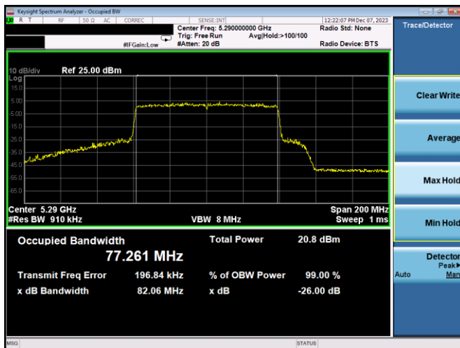
Plot 7-36. 26dB BW & 99% OBW Antenna WF8 (80MHz BW 802.11ax(SU) – Ch. 58, MCS4)
