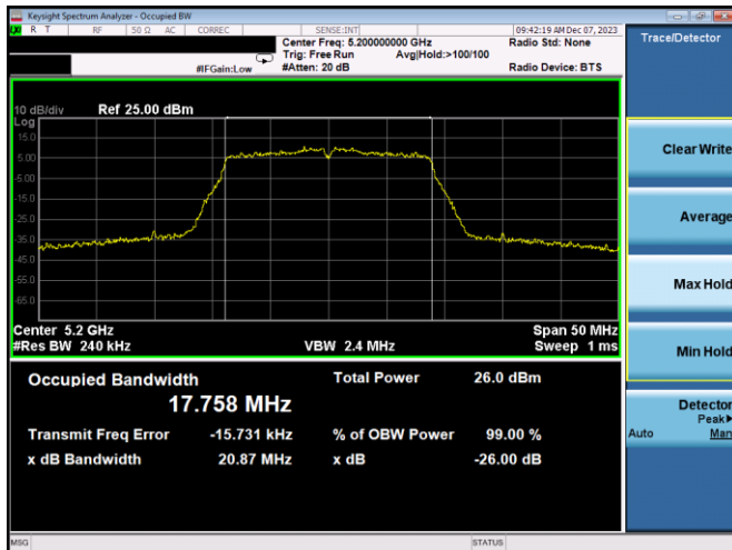
Plot 7-1. 26dB BW & 99% OBW Antenna WF8 (20MHz BW 802.11n – Ch. 40, MCS2)
