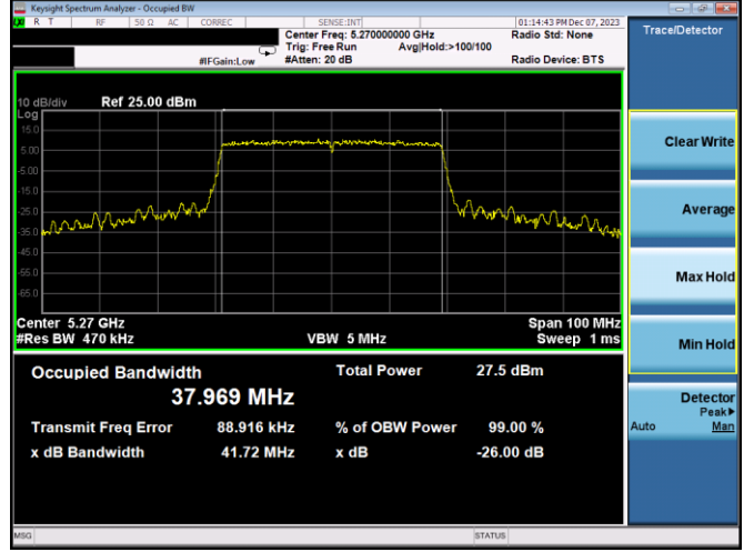
Plot 7-56. 26dB BW & 99% OBW Antenna WF8 (40MHz BW 802.11ax(SU) – Ch. 54, MCS11)
