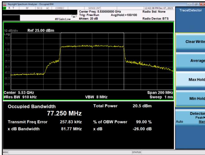
Plot 7-42. 26dB BW & 99% OBW Antenna WF8 (80MHz BW 802.11ax(SU) – Ch. 106, MCS4)
